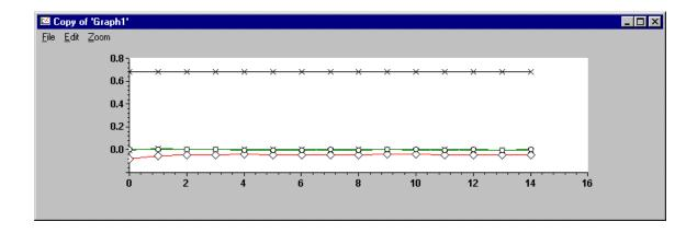
This is just an illustration of the need to allow for the KPCI-3108's faster acquisition time. The effect is a function of gain, sampling speed and the source resistance of the individual signals being measured. Application software that controls this combination of hardware needs to take this effect into consideration and quantify it for the particular situation in order to achieve maximum system accuracy.
