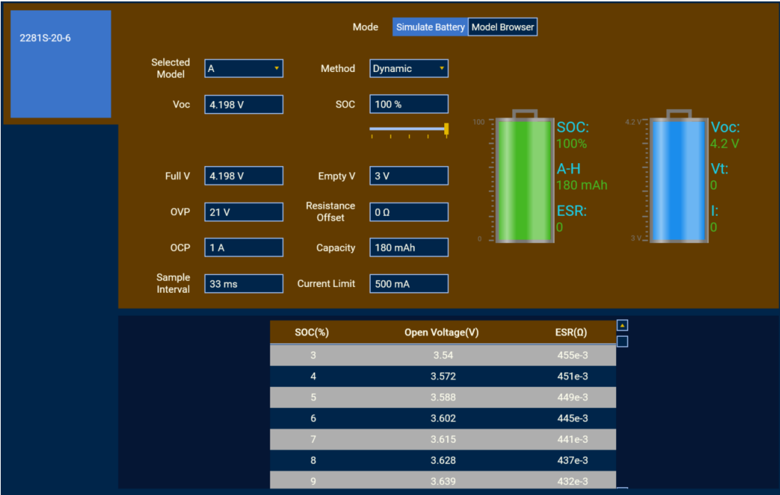
Figure 10: Simulate Battery in KickStart Software
