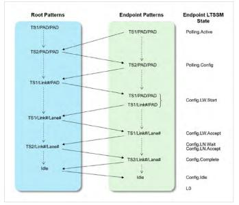
Figure 7. Link training sequence between RC and EP<sup>3</sup>.
