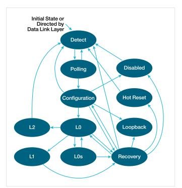
Figure 3. Link Training State Machine<sup>3</sup>.
