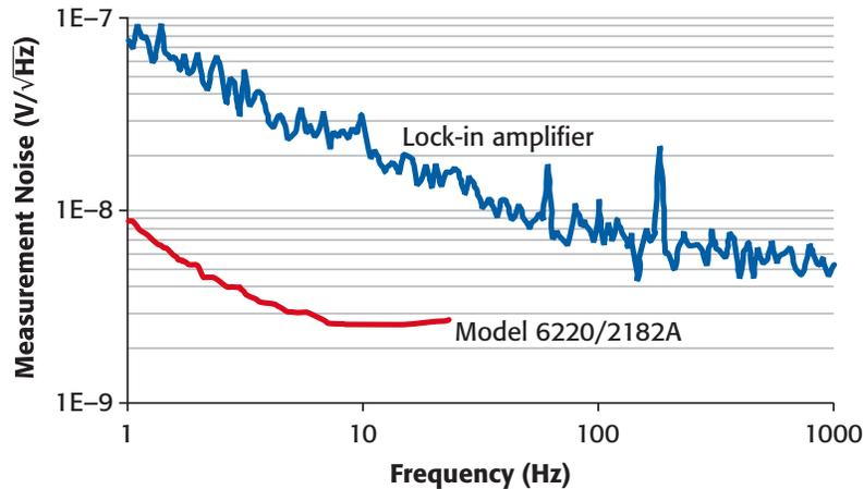
*Figure 7. Noise comparison of SRS 830 lock-in amplifier and DC reversal measurements with Keithley Models 6220 and 2182A.*
