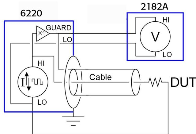
*Figure 6. Guard buffer circuit in a two-wire, DC reversal measurement.*
