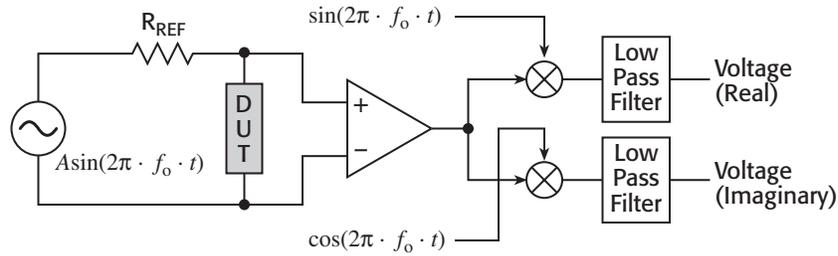
Figure 1. Simplified block diagram of a lock-in amplifier measurement setup.
