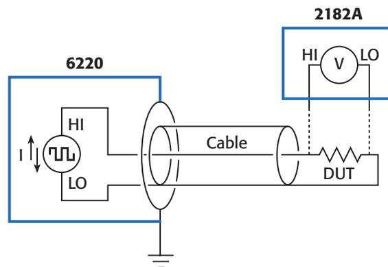
Figure 2. DC reversal measurement circuit using a four-wire lead arrangement.
