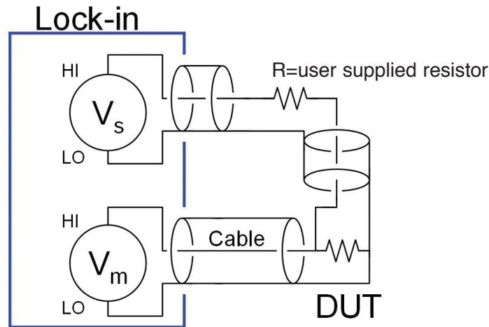
*Figure 5. Making a “current source” from a lock-in amplifier*
