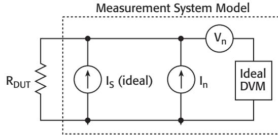
*Figure 9. Idealized measurement circuit with current and voltage noise sources,  $I_n$  and  $V_n$ .*
