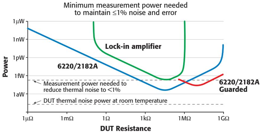
Figure 8. DUT power required for typical measurements with different instruments.
