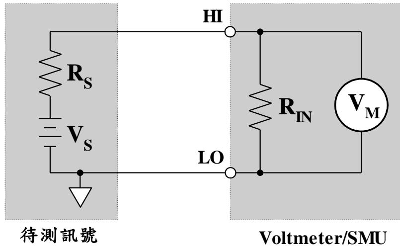
$$\text{量得電壓 } V_M = V_S \left( \frac{R_{IN}}{R_S + R_{IN}} \right)$$
