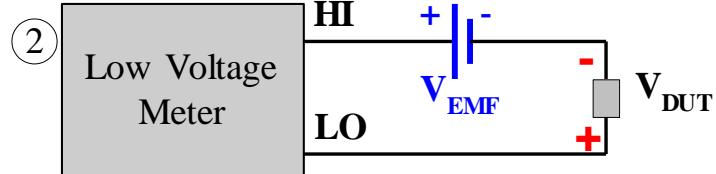
$$\frac{\text{Reading}\#1 - \text{Reading}\#2}{2} = \frac{(V_{\text{DUT}} + V_{\text{EMF}}) - (-V_{\text{DUT}} + V_{\text{EMF}})}{2} = V_{\text{DUT}}$$
