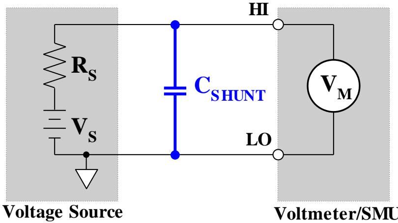
$$\text{量得電壓} = V_S(1 - e^{-t/R_S C_{SHUNT}})$$
