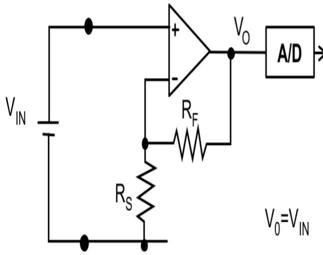
$$V_0 = V_{IN} \left[ \frac{R_S + R_F}{R_S} \right]$$
