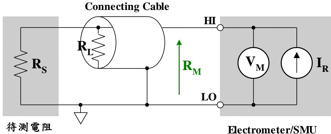
$$\text{量得電阻 } = R_M = R_S \left( \frac{R_L}{R_S + R_L} \right)$$
