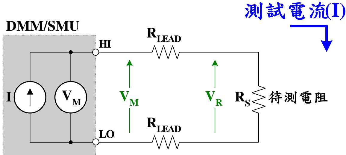
$$\text{量得電阻} = \frac{V_M}{I} = R_S + (2 \times R_{LEAD})$$
