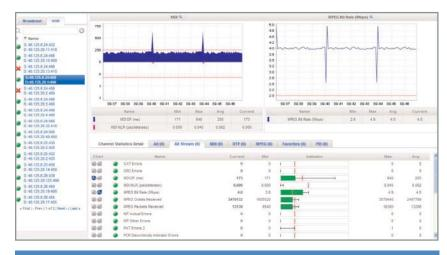
Access real-time statistics through a user friendly, web-based GUI for a comprehensive view of all Broadcast and VoD channels. Tektronix' IP Video solution offers statistics by location and by use, channel summaries and detailed statistics and alarms with real-time graphing.
