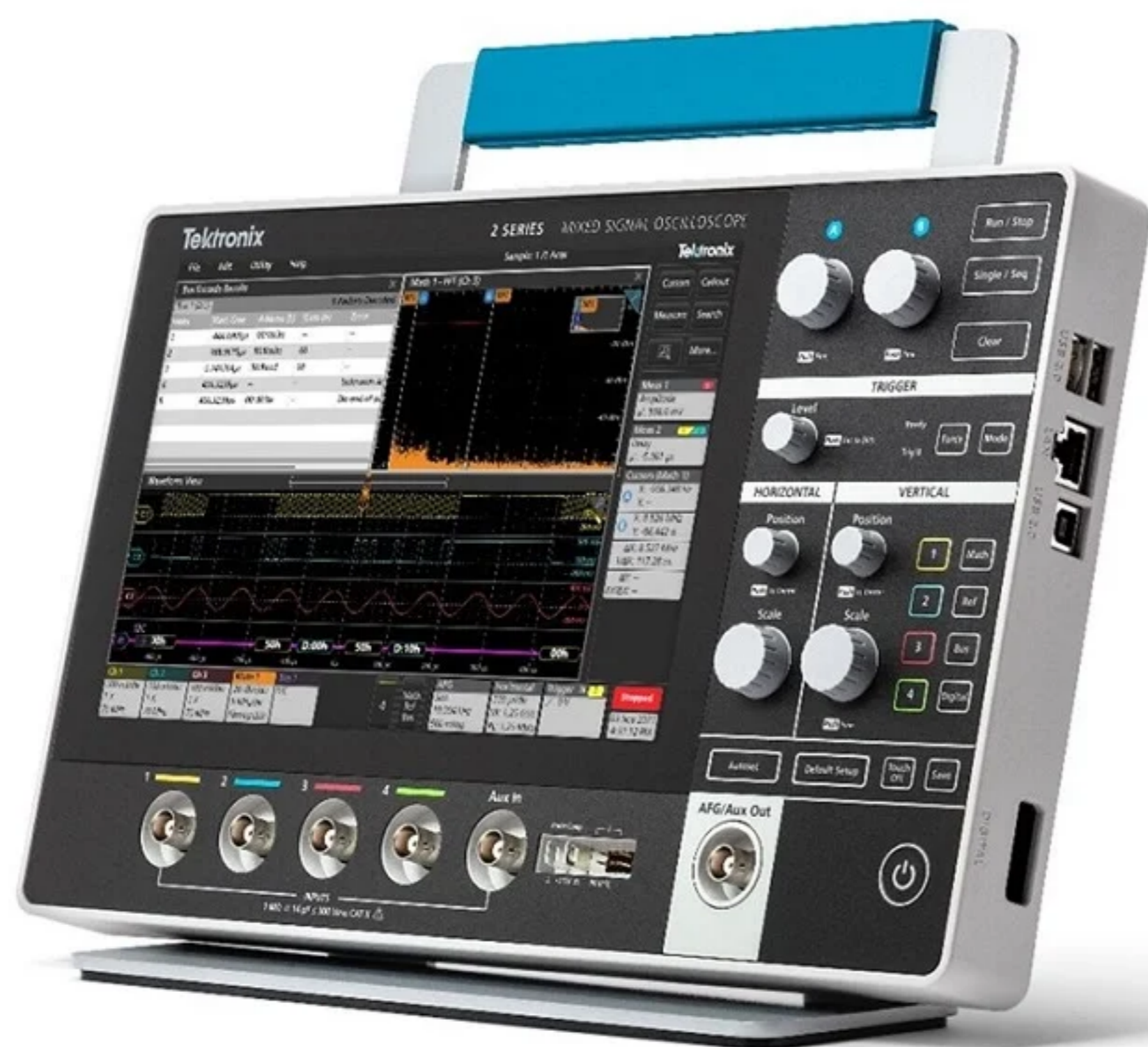
This 2 Series Mixed Signal Oscilloscope boasts a 1.5-in form factor and a weight under 4 pounds. Source: Tektronix Inc.
