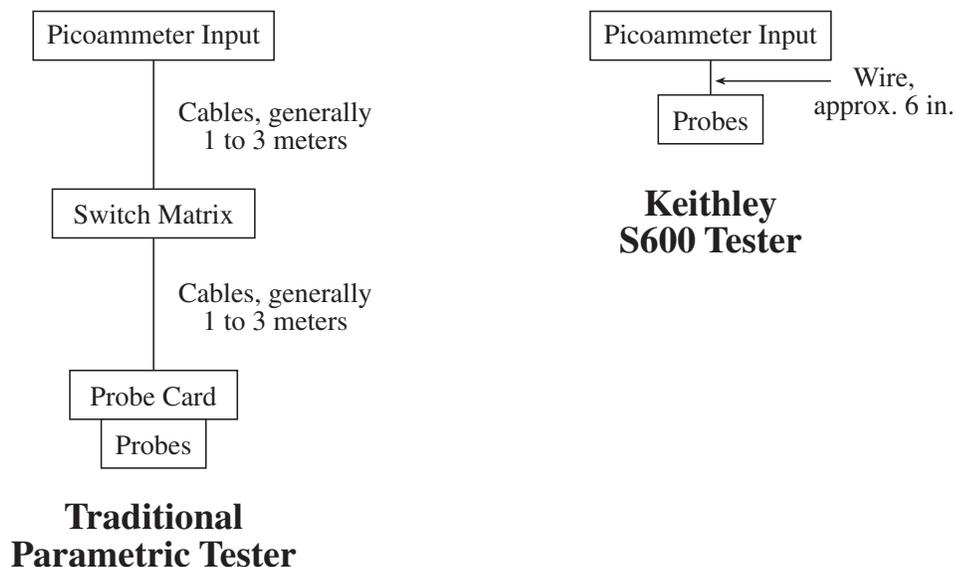
**Figure 2.** Reducing the length of the signal path between the probes and picoammeter input reduces the test’s parasitic dielectric absorption effect and allows measuring the dielectric absorption effect on a typical test structure.
