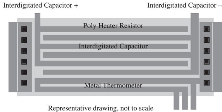
**Figure 3.** Self-heated capacitor for  $\kappa$  drift measurements for low  $\kappa$  ILD material
