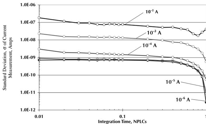
**Figure 9.** The standard deviation of current measurements vs. NPLCs (integration time) of the 2400 SourceMeter instrument for the 10<sup>-2</sup>, 10<sup>-3</sup>, 10<sup>-4</sup>, 10<sup>-5</sup>, 10<sup>-6</sup> measurement ranges
