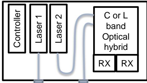
**OM4006\ OM4106** Base product is either C or L band. Laser 2 is internally connected for use as the Reference Laser (LO).
