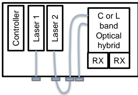
**EXT** Modifies base product to allow use of external laser for Reference Laser (LO). Includes armored PM jumper cable for use of internal laser.
