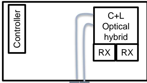
**OM4006\ OM4106 NL** Base C+L receiver for operation over C+L (1530 to 1610nm). No lasers are included in base C+L model.
