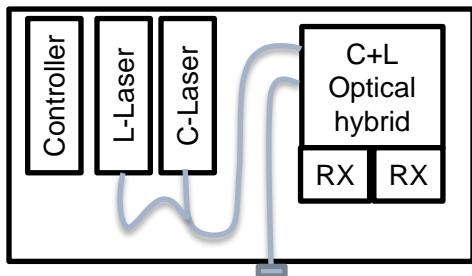
**OM4006\ OM4106 CL** Modifies base C+L product to include 1 C and 1 L band laser internally coupled to the Optical Receiver
