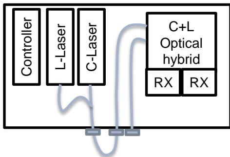
**EXT** Modifies base product to allow use of external laser for Reference Laser (LO). Includes armored PM jumper cable for use of internal laser.
