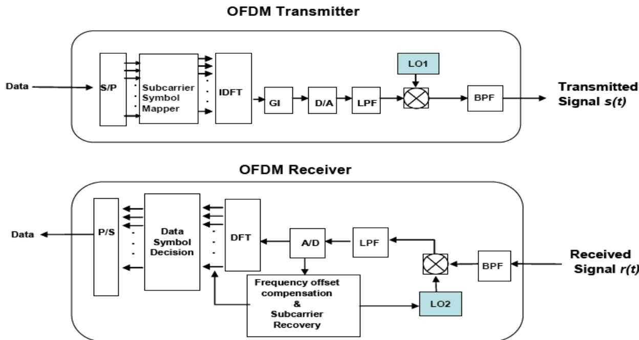
S/P: Serial-to-parallel    GI: Guard Time Insertion    D/A: Digital-to-Analog    (I)DFT:
