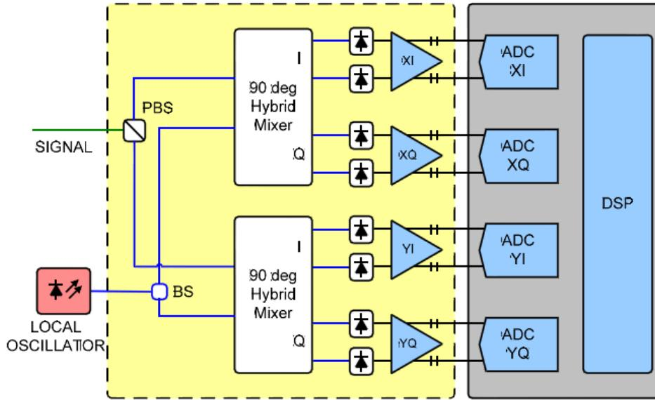
Replace ADC with real-time oscilloscope
