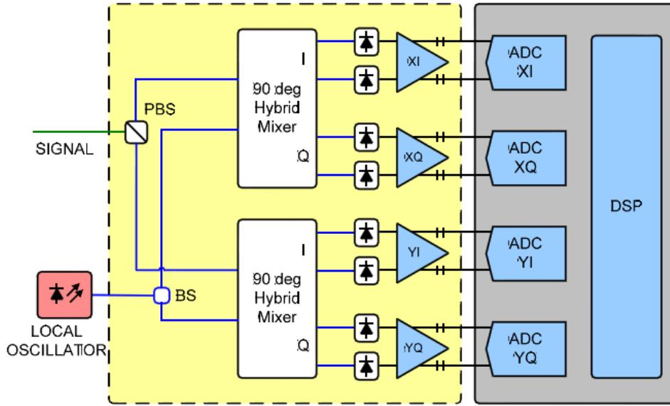
Replace ADC with real-time oscilloscope
