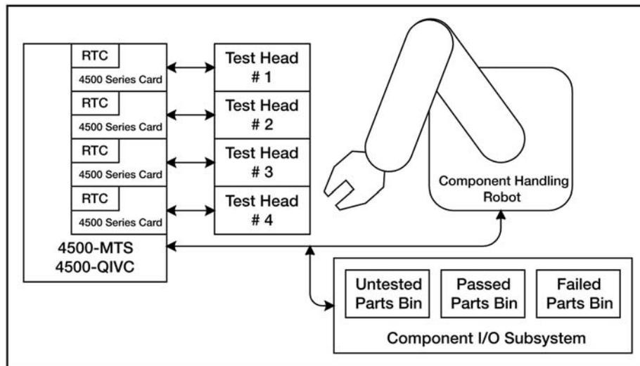
**Figure 1.** Real-time controller cards make true asynchronous concurrent testing a reality. While the RTCs execute tests, other test system resources are free to command the component I/O and robotic handling subsystems.
