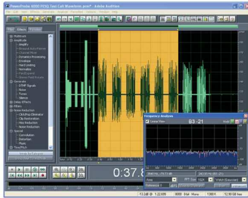
With the DirectQuality R7 Web Interface you can launch off-the-shelf tools such as Adobe® Audition to perform deep speech waveform frequency and time-domain analysis on recorded PESQ samples.
