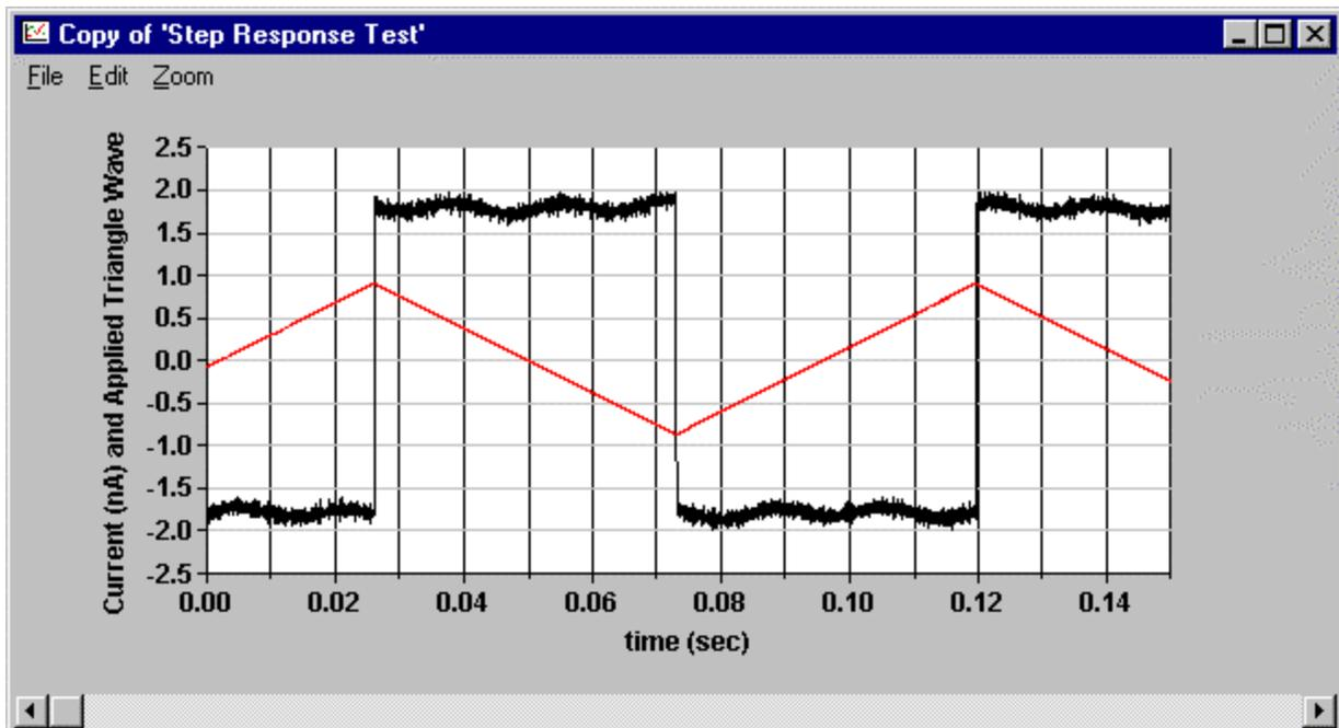
However, the 428 has some very flexible filtering options as the next graph shows. In this case, the applied signal is unchanged, but the programmable rise time filter feature was turned on. A rise time of 1 msec was used. As can be seen, the noise is reduced but at the expense of response time. Even so, these data clearly demonstrate the superior response time of the 428 current amplifier for situations where measurement of a rapidly changing signal is the primary goal.
