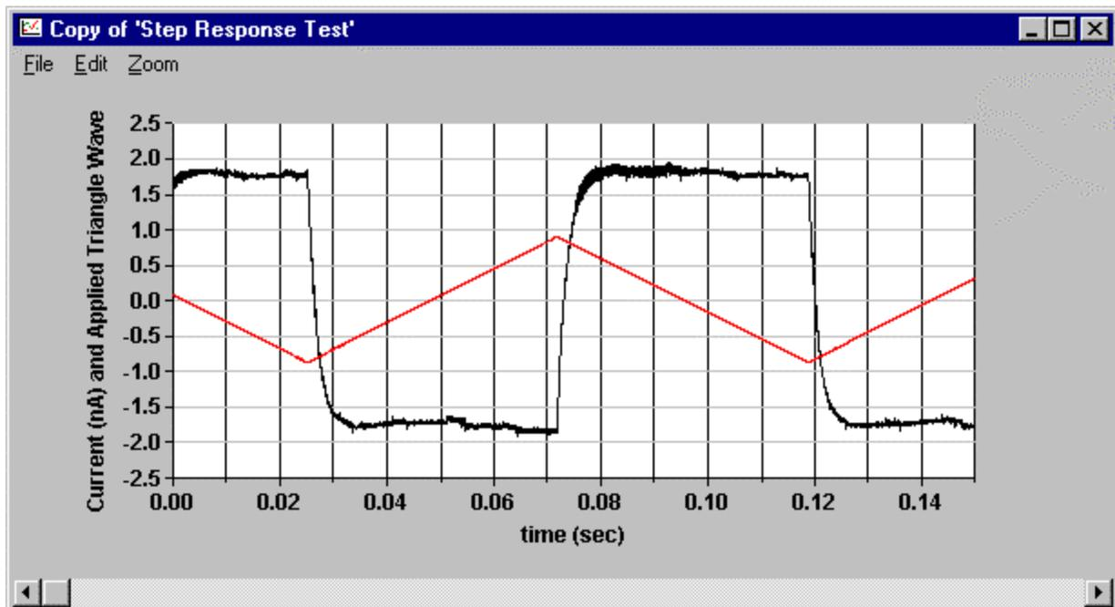
Below are data from a model 6485 picoammeter. The picoammeter was on the 2nA range; filtering was OFF. As the graph demonstrates, similar to the results with the 6487, there is a significant response time. The response time of the 6485 is longer than for the 6487.
