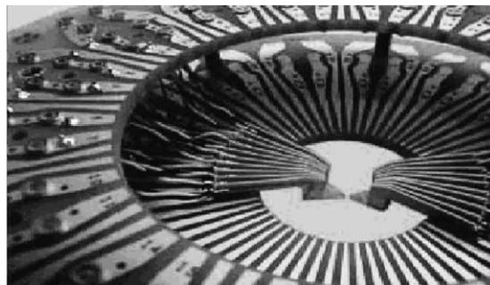
**Figure 4.** Keithley S600 Series low leakage probe card.
