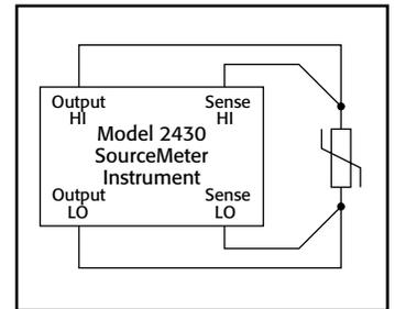
**Figure 9. Four-wire connection.**
