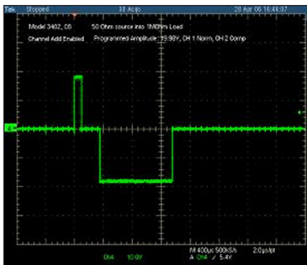
Figure 3. Write/Erase pulse train used for flash memory testing, and created with a PG's channel-add feature.
