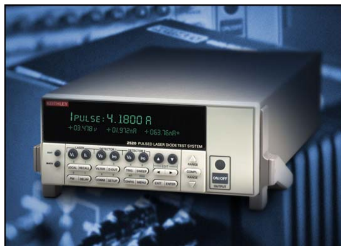
Figure 7. It is possible to put all the functionality shown in Figure 6 in a pulsed source-measure unit (the Keithley Model 2520 pulse laser diode test system) with output impedance and cabling that closely matches the impedance of the laser diode. The measurement portion of the system incorporates multi-channel data acquisition, dedicated timing circuitry, high speed current-to-voltage converters, and a digital signal processor (DSP) that emulates DSO functionality and controls much of the measurement sequence.
