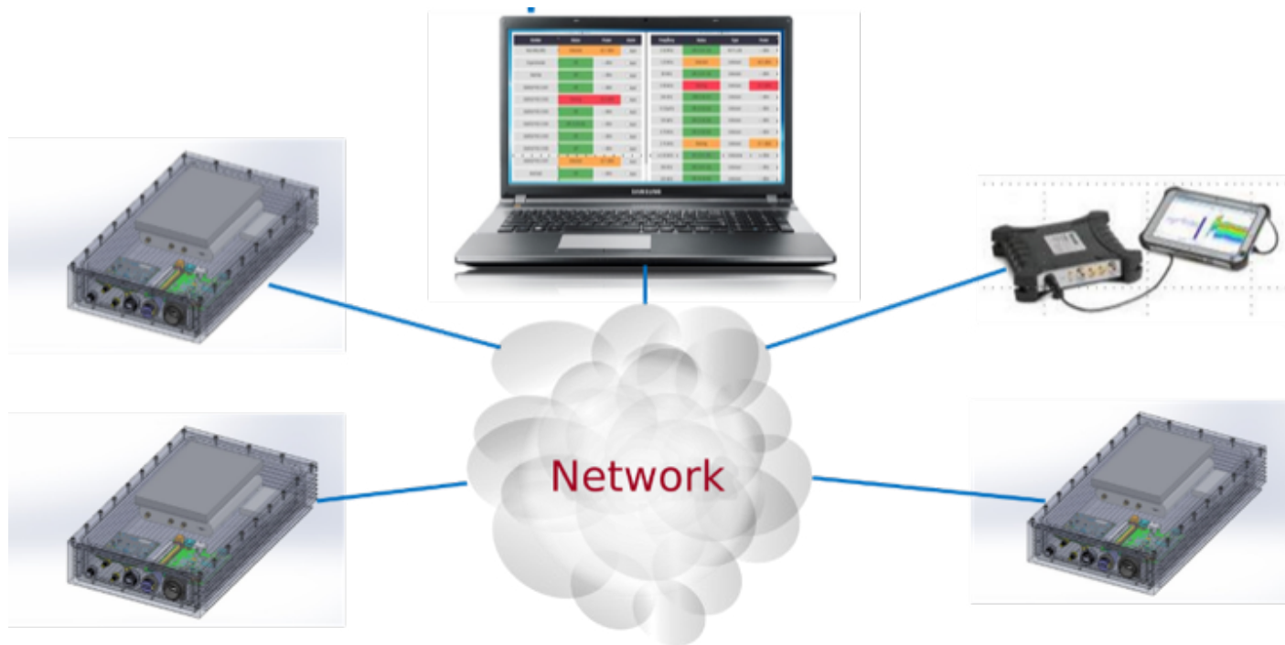
FIGURE 5. Tektronix USB Real-Time Spectrum Analyzers support network-ability to create a high performance, intelligent RF sensor network.
