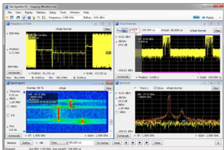
These acquisitions can range from a few microseconds to several seconds or more, depending on settings and hardware used. This type of capture, analysis and replay is supported by all of the real-time spectrum analyzers, as well as offline analysis with SignalVu-PC software.
