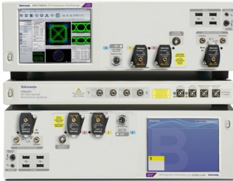
*Figure 12: Coherent optical configuration showing the DPO70000SX system where one unit is inverted so ATI ports can be located near the optical receiver in the middle to preserve signal fidelity.*
