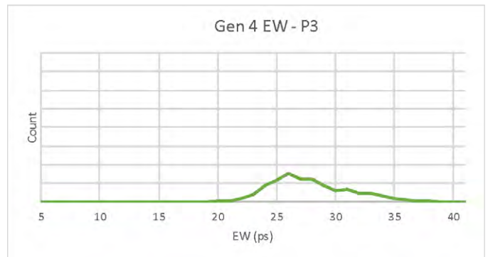
Distribution by PCIe Preset 3 for Gen 4 Eye Width – AICs Only.
