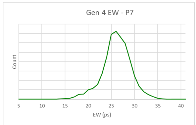
Distribution by PCIe Preset 7 for Gen 4 Eye Width across all devices tested.
