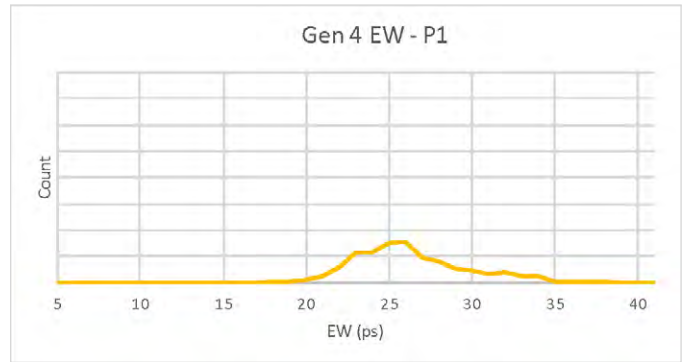
Distribution by PCIe Preset 1 for Gen 4 Eye Width – AICs Only.
