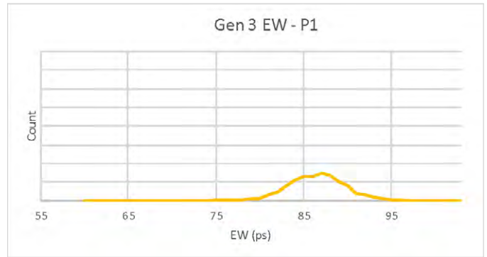
Distribution by PCIe Preset 1 for Gen 3 Eye Width – AICs Only.
