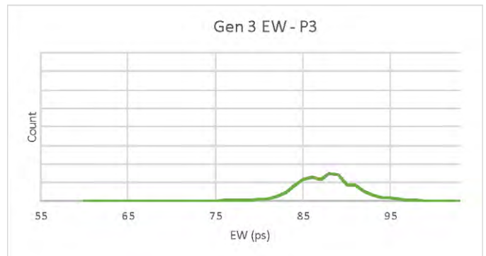
Distribution by PCIe Preset 3 for Gen 3 Eye Width – AICs Only.
