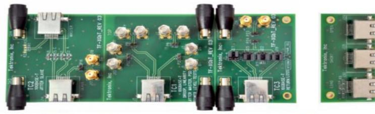
Fig 1: XGbT Test Fixture main board
