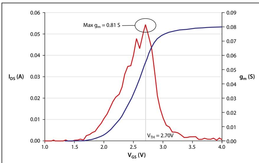
Figure 3B.  $g_m$  test with optimal cabling and grounding. From this measurement,  $g_m$  is 0.81 S and  $V_{TH}$  is 2.70V.
