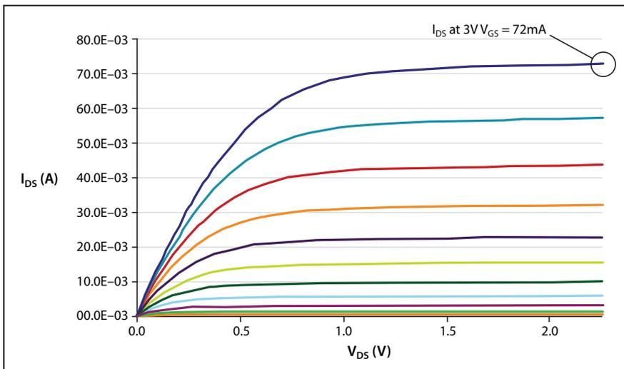
Figure 2B. MOSFET curves with optimal cabling and grounding.  $I_{DS}$  at a  $V_{GS}$  of 3V is measured as 72mA.
