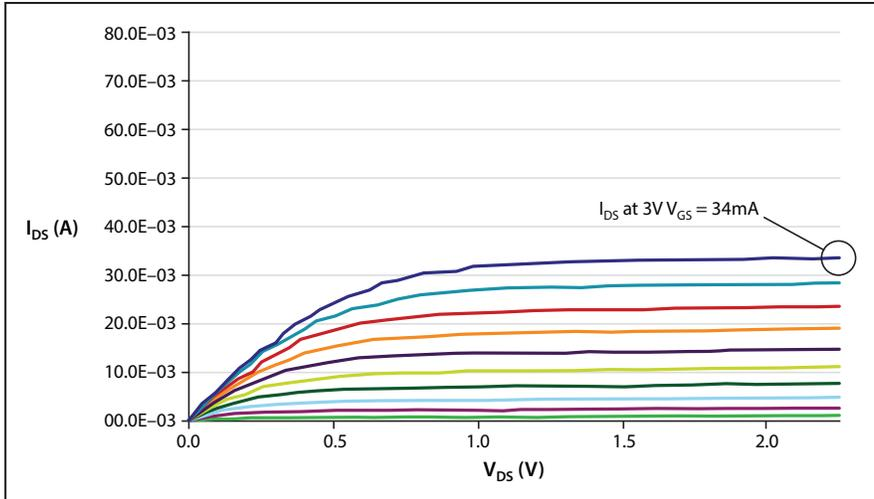
Figure 2A. MOSFET curves with poor cabling and grounding.  $I_{DS}$  at a  $V_{GS}$  of 3V is measured as 34mA.
