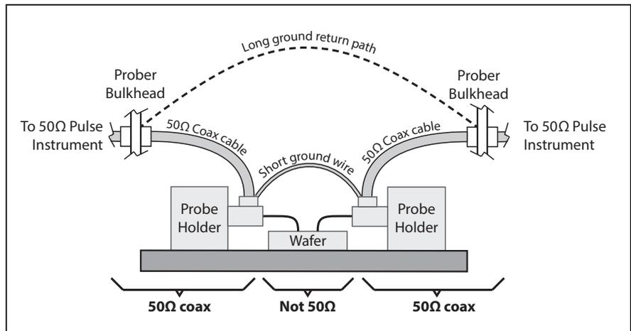
Figure 1. Probe hookups usually do not maintain 50Ω all the way to the DUT. If the short ground wire is not used, the much longer ground return path will limit bandwidth.
