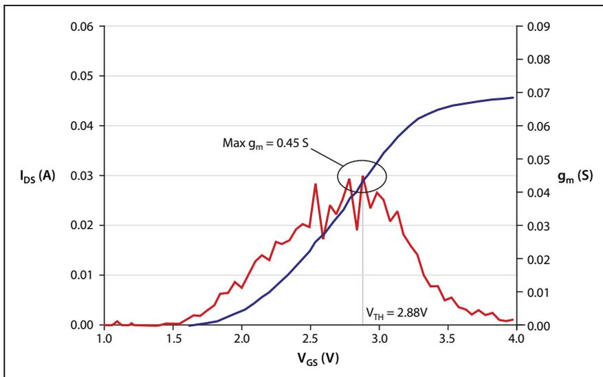
Figure 3A.  $g_m$  test with poor cabling and grounding.
