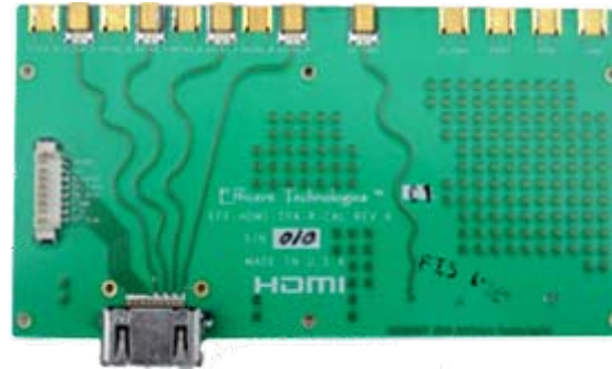
TPA-R (Receptacle fixture with TDR calibration traces)
