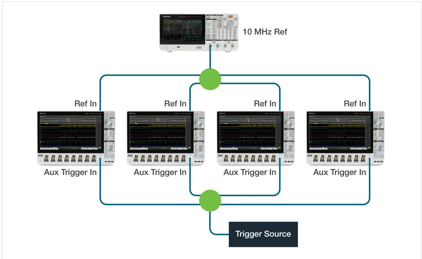
**Figure 3.** In this system, both the Aux Trigger inputs and timebase references are fed by splitters and matched 50  $\Omega$  cables. This setup gives the best skew results without sacrificing a channel from each oscilloscope. Using input channels instead of the Aux Trigger inputs will reduce the number of measurement channels, but will reduce trigger jitter by about 200 ps.
