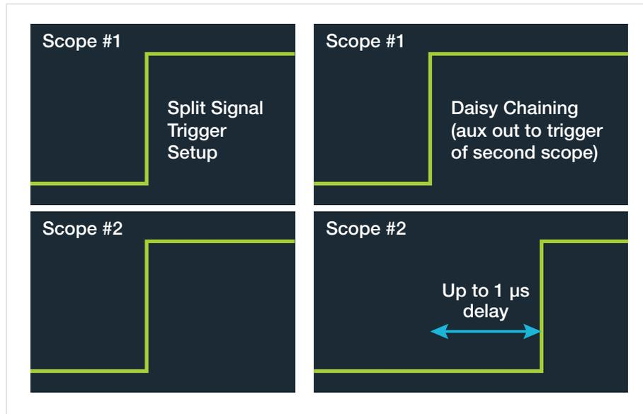
Figure 2. Different trigger setups result in different skew or delays. The setup on the left uses two oscilloscopes with phase matched cables feeding each instrument's trigger channels. The setup on the right shows the impact of "daisy chaining", in which one oscilloscope's Aux output feeds the next oscilloscope's trigger channel. Daisy chaining can cause significant delays.
