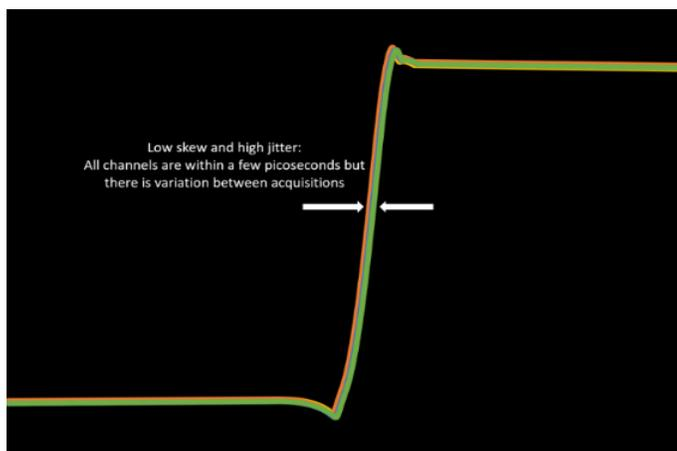
Figure 1c: Low skew & high jitter.
