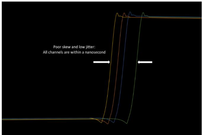
Figure 1b: High skew & low jitter.
