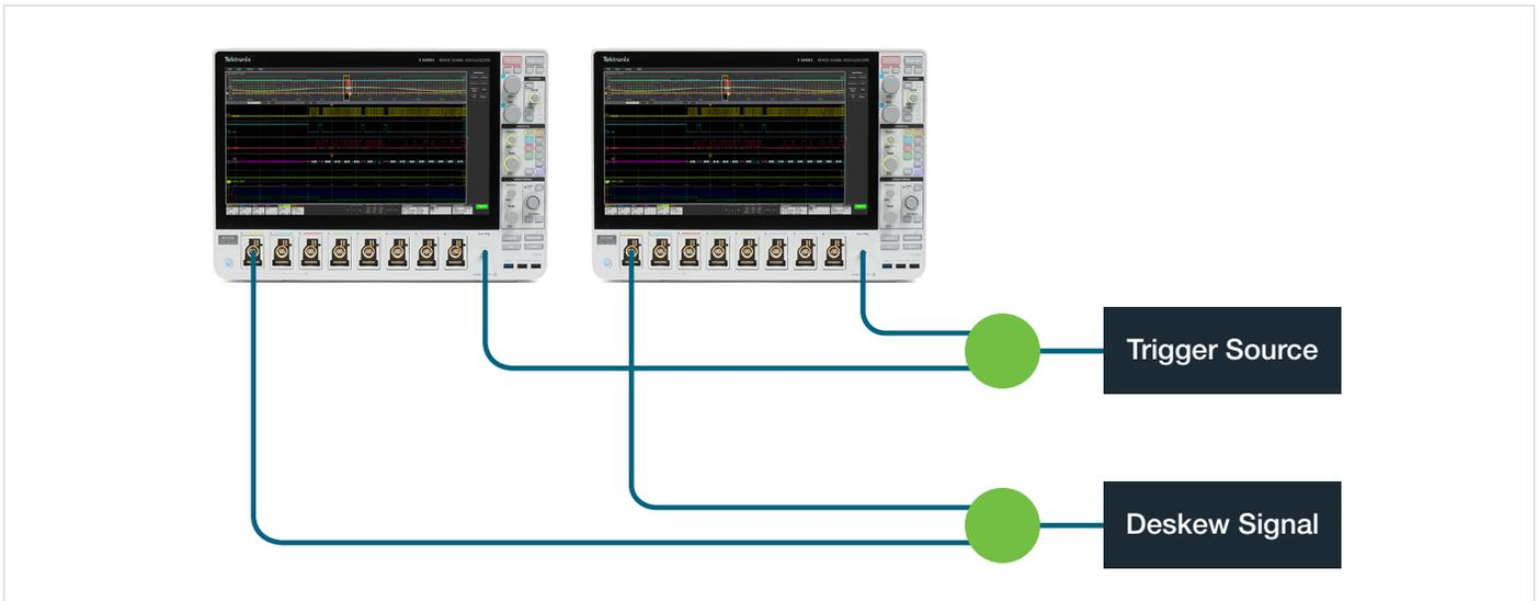
Figure 13. For the deskew process, a clock signal that is not the trigger signal should be applied to the two channels being deskewed. Here the trigger signal is being split into the Auxiliary Inputs and the deskew signal is being split into Channel 1 on each oscilloscope.
