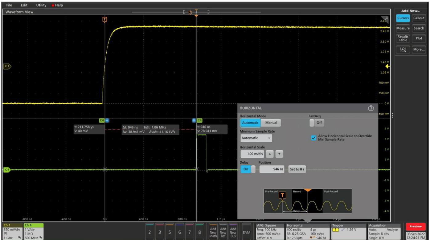
Figure 9. CH1 is the trigger source. CH4 is the Aux trigger out. The measured 946 ns skew is removed using pre trigger delay.
