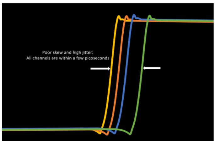
Figure 1d: High skew & high jitter (worst).
