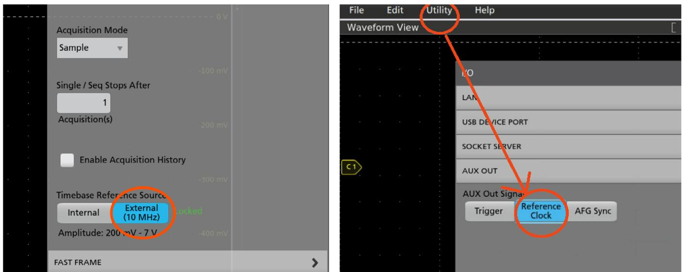
Figure 6. 5 and 6 Series MSO menus for setting up the reference clock and locking the timebase reference. The left side shows the settings for setting the timebase reference on a receiving oscilloscope. The right side shows the settings for setting the Aux Out to output the reference clock on a transmitting oscilloscope.
