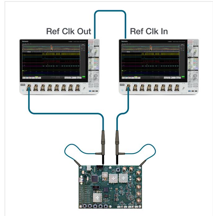
**Figure 7.** When using “double-probing” to synchronize two oscilloscopes, each oscilloscope must have the same trigger parameters and the probes must be identical. The baseline skew should be low enough to be corrected with Deskew controls.
