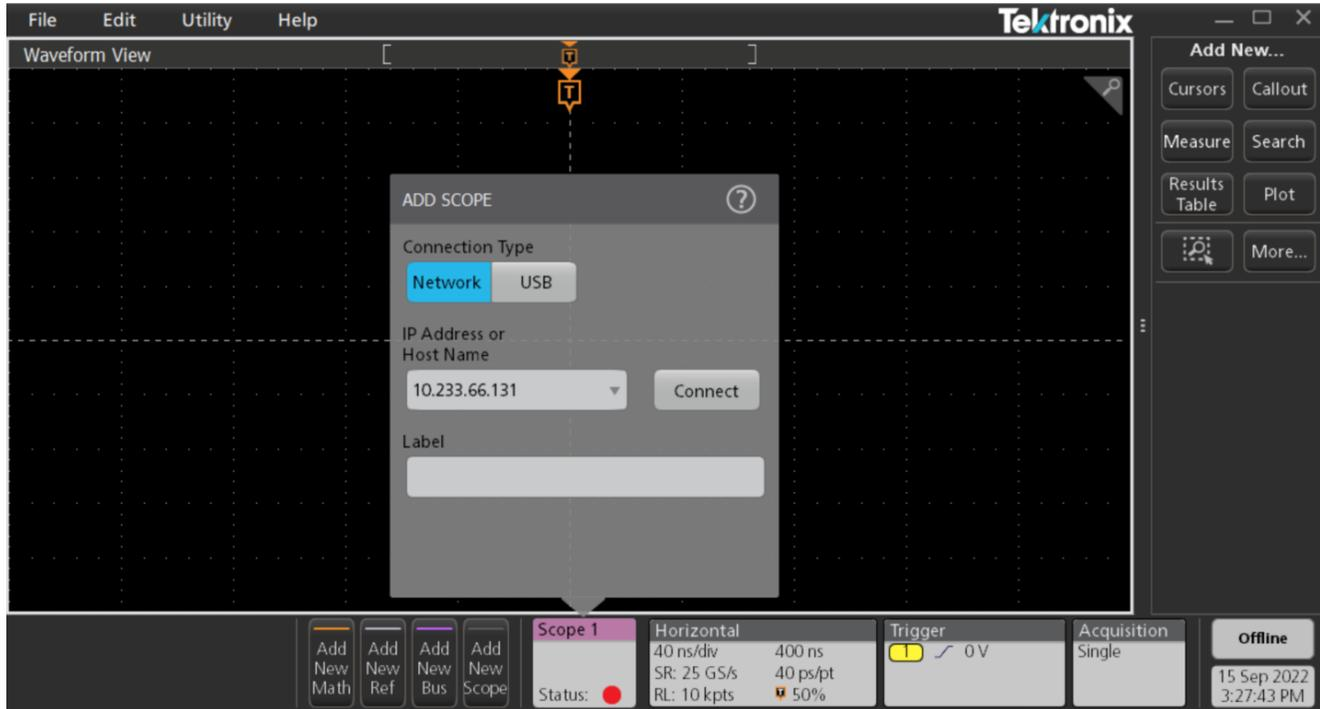
Figure 11. Adding an additional oscilloscope connection with the “Add New Scope” badge in TekScope PC.
