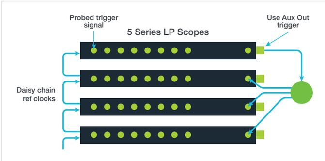
Figure 8. If the skew requirements are not absolutely critical, one can use a trigger on a master oscilloscope and split Aux Out to trigger additional oscilloscopes.
