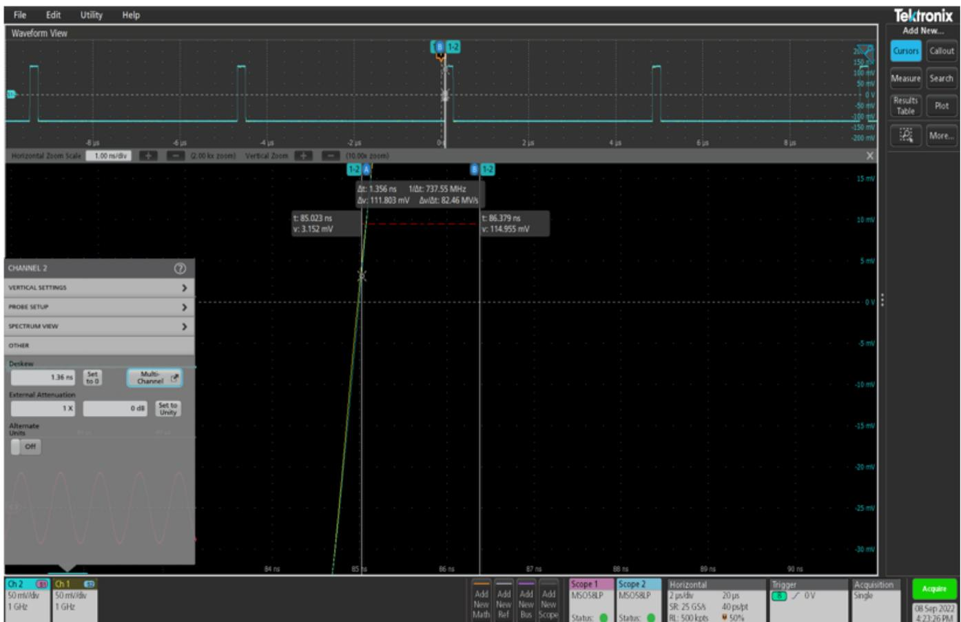
Figure 17. Entering the measured delta time in the Deskew setting in the channels vertical badge will correct for the skew between the two channels.
