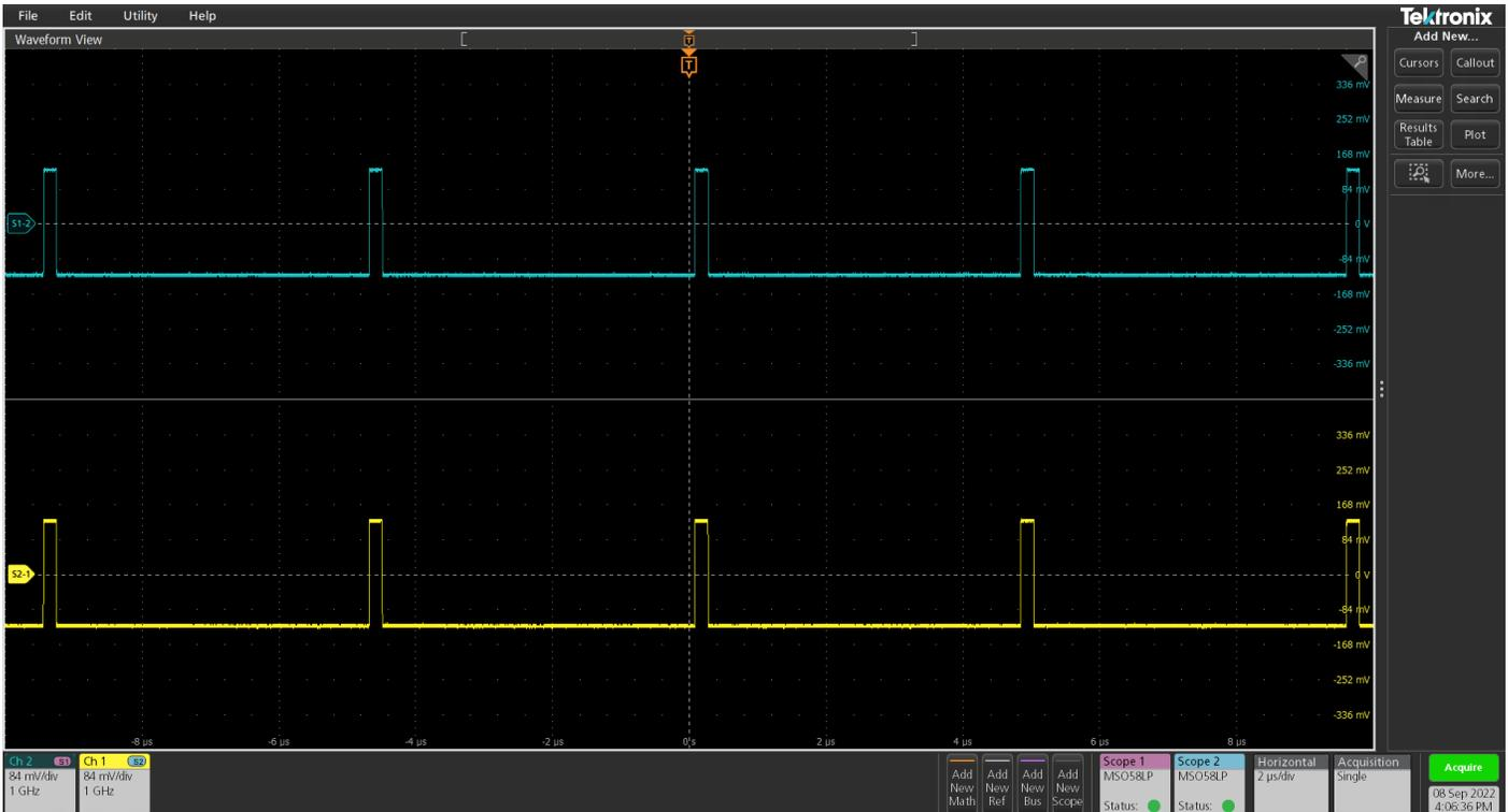
Figure 14. Same signal applied to the two channels being deskewed.
