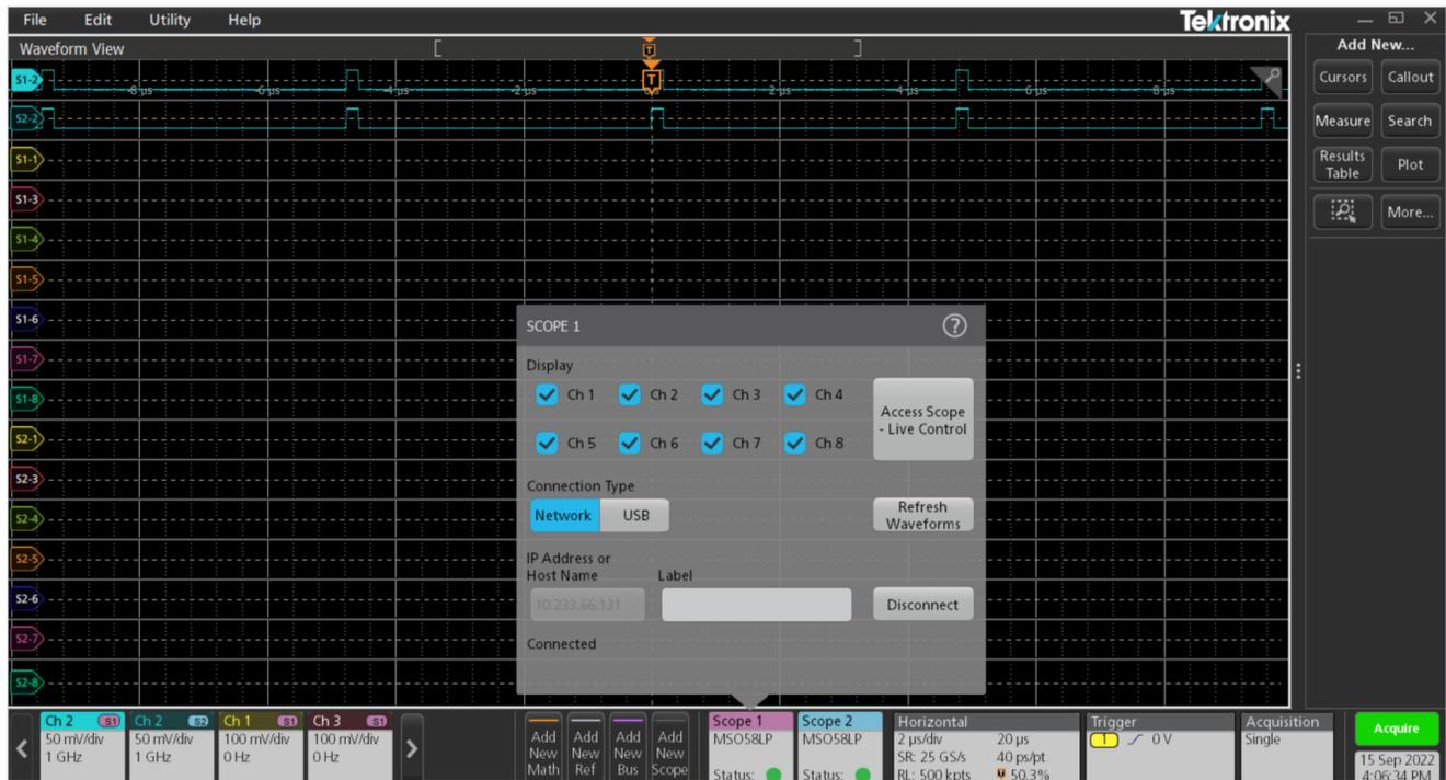
Figure 12. Additional channels are displayed or hidden after the scope is connected.
