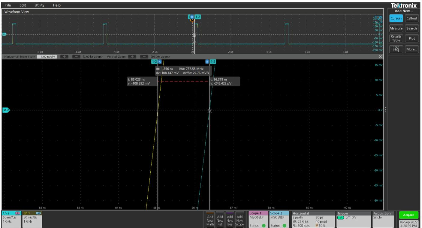
Figure 16. Measuring the delta time between two channels on different scopes.
