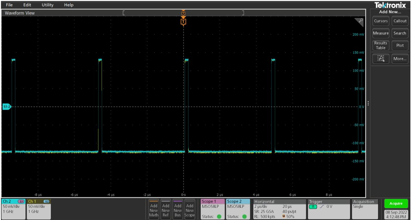
Figure 15. Signals to be deskewed are zoomed in and displayed in overlay mode.
