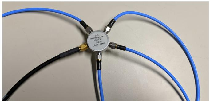
**Figure 4.** An SMA power splitter connected to four matched cables and a trigger source
