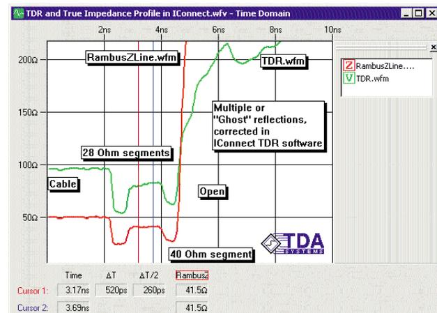
Figure 9. TDR and true impedance profile for the Rambus notebook module. Each segment of the true impedance profile can be correlated to a physical structure in the module trace. Multiple reflections in TDR waveform are corrected in IConnect to produce an accurate impedance measurement
