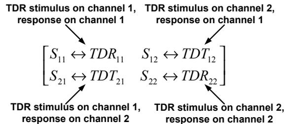
**Figure 4. There is a clear relationship between TDR and TDT measurements in time domain and network analyzer measurements in frequency domain**
