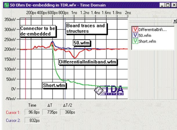
**Figure 14. De-embedding of the probe effects by subtracting the reference 50-Ohm waveform. One can clearly see that we can remove the probe connector effects by subtracting the 50-Ohm reference waveform from the DUT and reference short waveforms**
