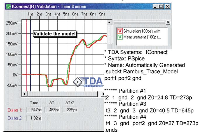
**Figure 11. Correlation between simulation of the interconnect modeling produced in IConnect TDR software and the original TDR measurement. Such good correlation at 45 ps rise time of the TDR oscilloscope indicates excellent accuracy of the model**
