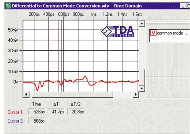
**Figure 16. Differential to common mode conversion in IConnect TDR software. The segments where the common mode is generated from the differential stimulus will be the main EMI sources in this differential pair**
