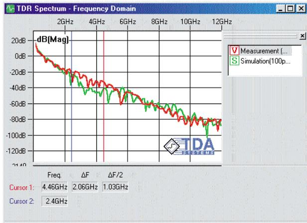
**Figure 12. Correlation between the spectra of the same two waveforms shown in Figure 11. There is as much as 1-2 dB of discrepancy at 2.5 GHz. However, this discrepancy is not significant enough to have an effect on the time domain measurement**
