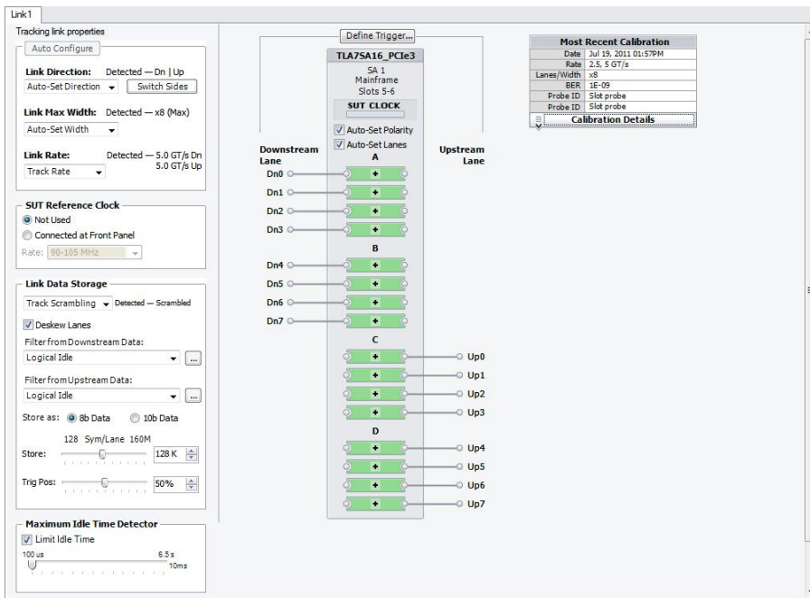
Figure 3. The LPA Setup window showing a successful configuration of a x8, 5.0GT/s link.
