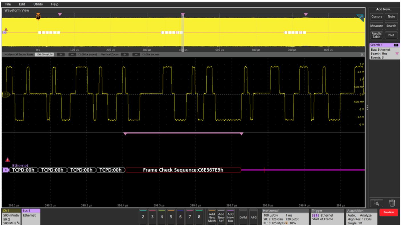
The decoded bus display above shows that three bursts of bus activity were captured. To find specific values in the activity, you can use Wave Inspector automatic search to mark each specified event. In this example, the automated bus search is configured to find all Frame Check Sequence errors and it shows 3 events, at the end of each burst of bus activity.
