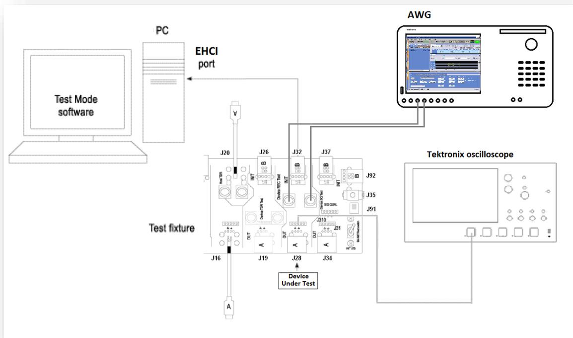
Figure 30: Equipment Setup for Receiver Sensitivity
