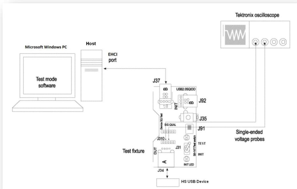
Figure 14: Equipment Setup for Suspend Measurement
