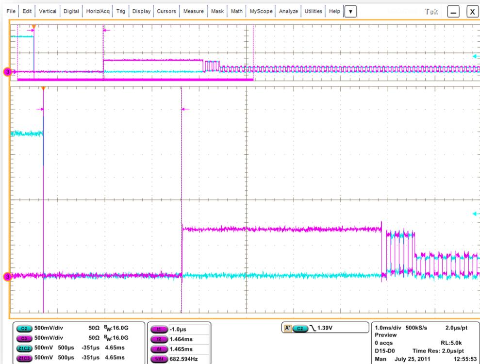
Figure 27: Device Chirp-K Latency (EL\_29)
