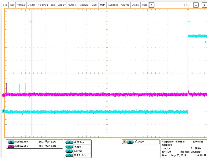
Figure 16: Device Response to Suspend from High-Speed
