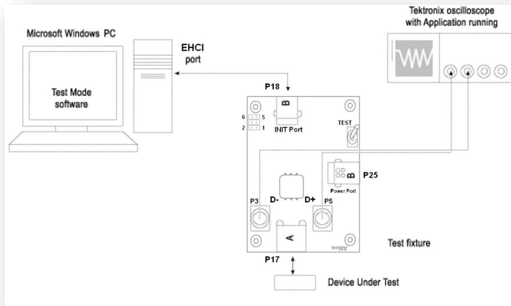
Figure 1: Equipment Setup for Signal Quality Measurement
