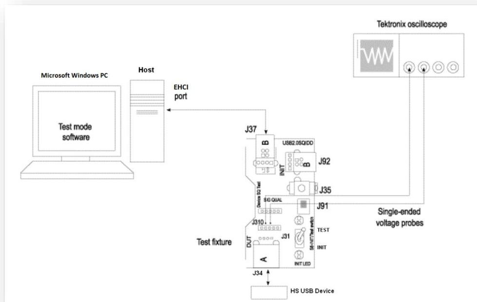
Figure 26: Equipment Setup for Chirp Measurement
