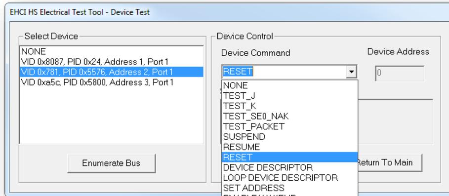
Figure 21: Device Reset
