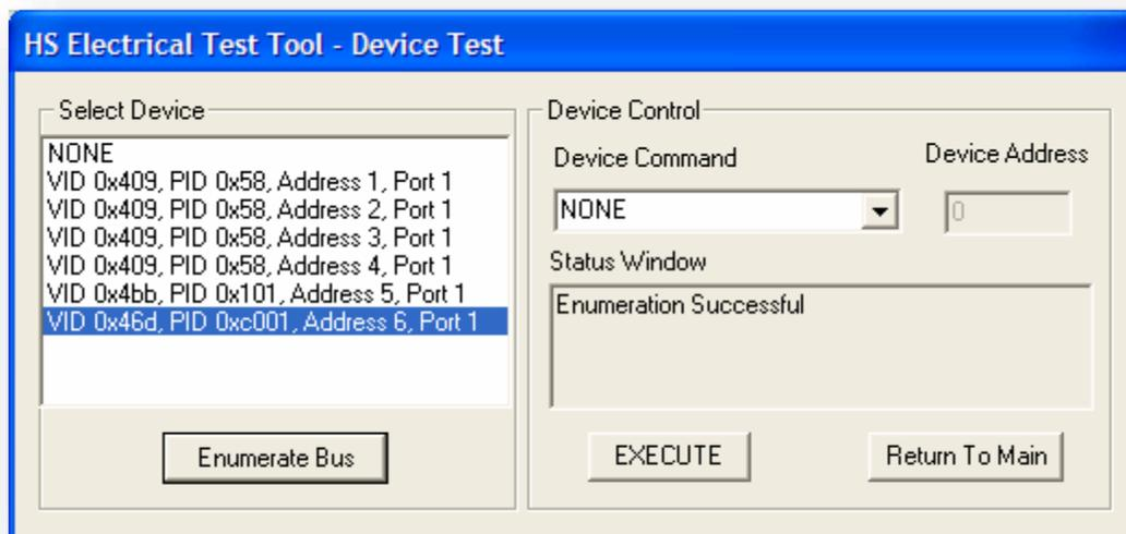
Figure 35: Full-Speed Electrical Test Tool Enumeration
