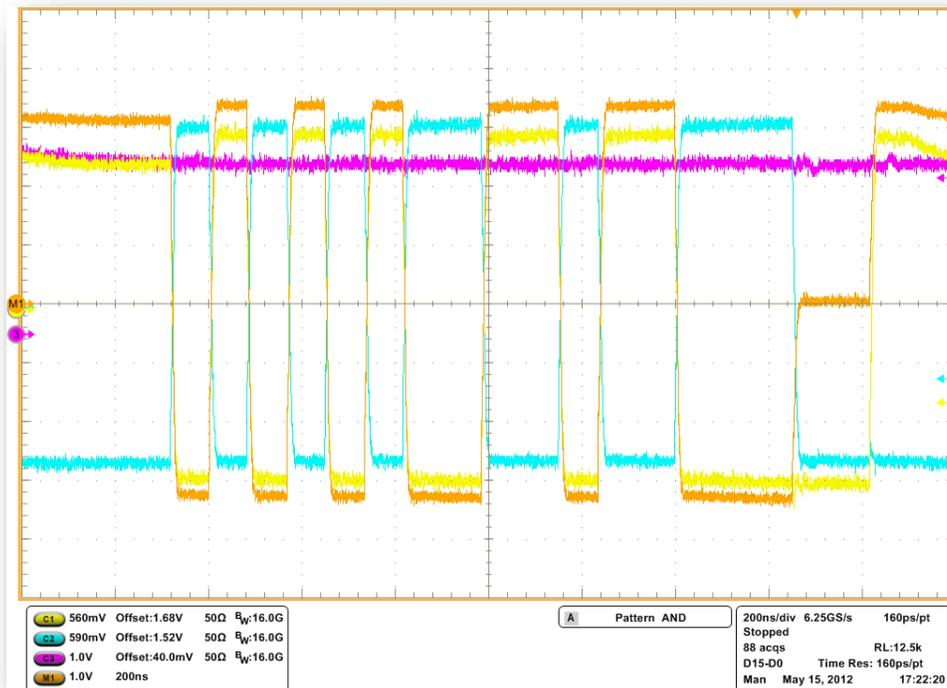
Figure 37: Full Speed Signal Quality trigger
