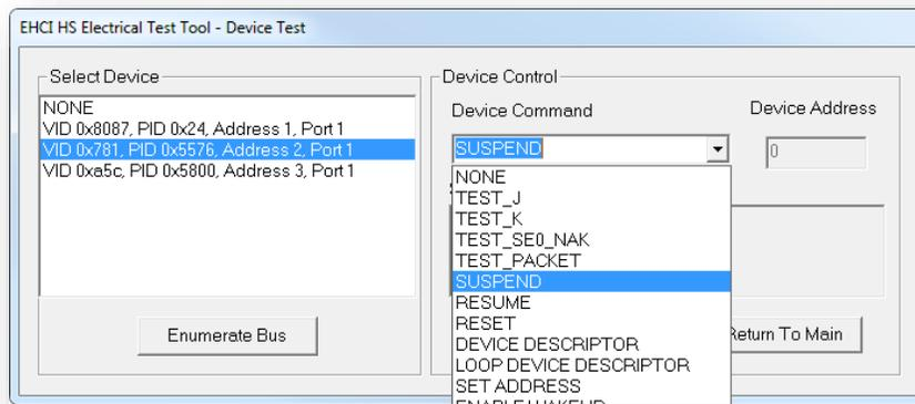
Figure 15: Device Suspend
