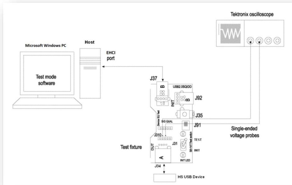
Figure 23: Equipment for Reset from Suspend Measurement
