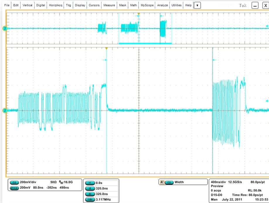
Figure 9: EL\_22 Device inter-packet gap
