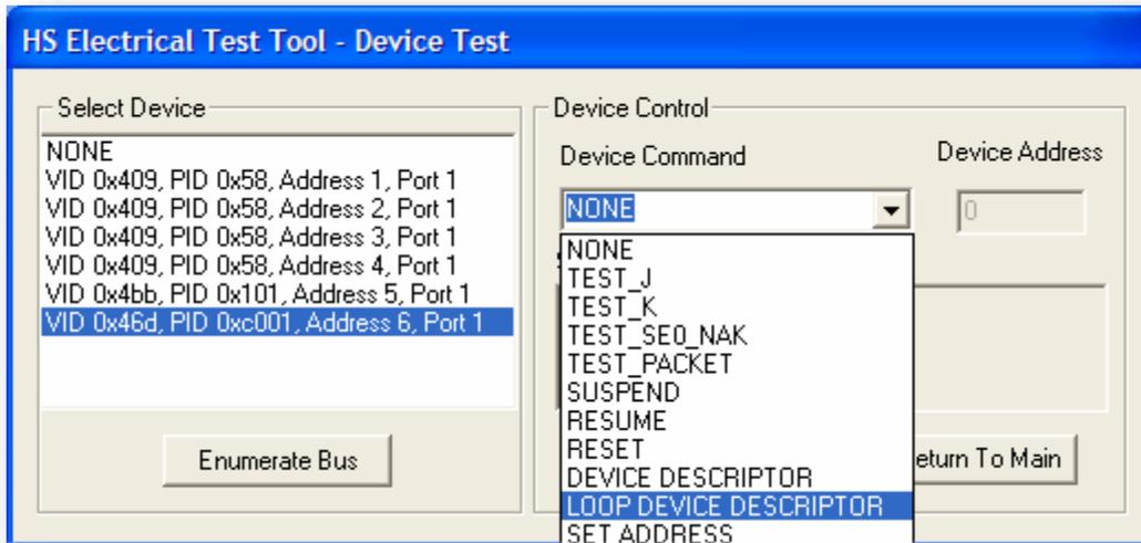
Figure 36: Loop Device Descriptor for Signal Quality Full Speed (Upstream)
