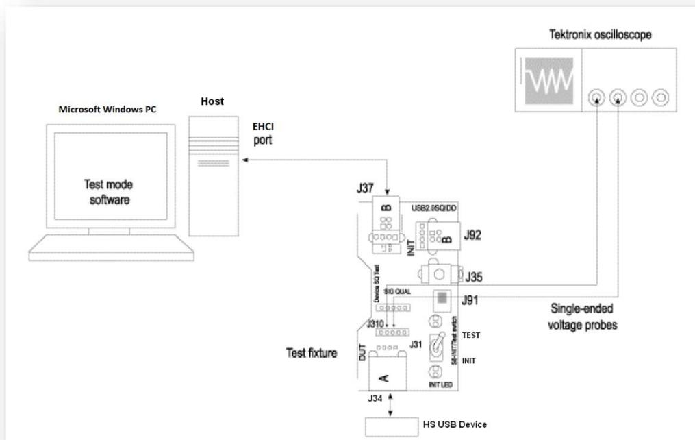
Figure 17: Equipment Setup for Resume Measurement
