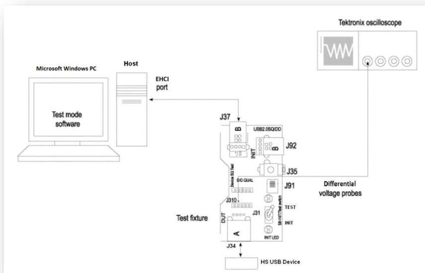
Figure 7: Equipment Setup for Packet Parameter Measurement
