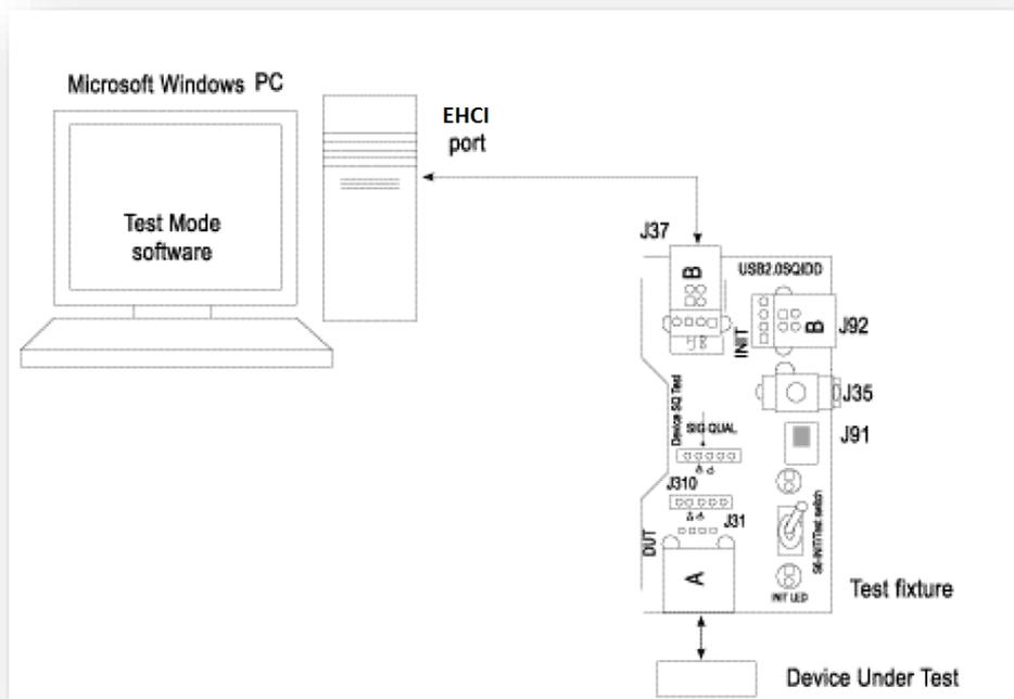
Figure 28: Equipment Setup for J/K, SE0\_NAK Test
