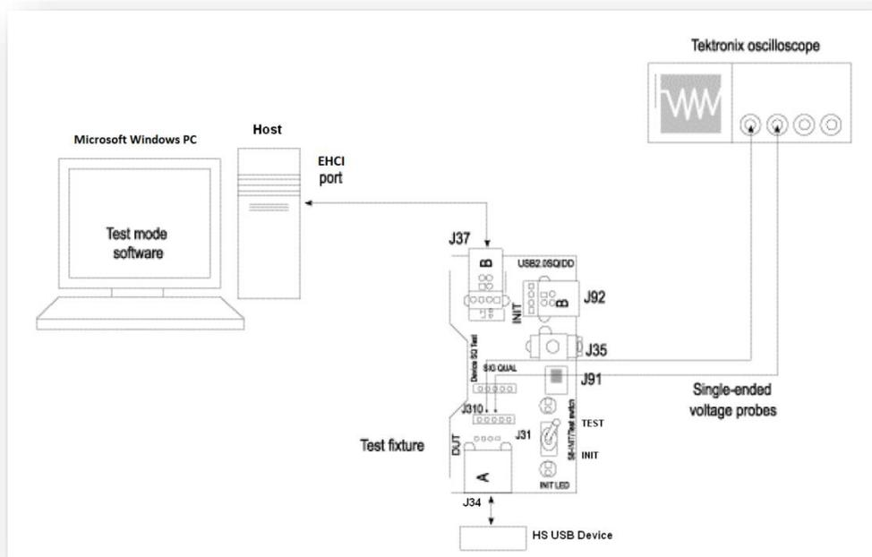
Figure 20: Equipment Setup in Reset from High Speed Measurement
