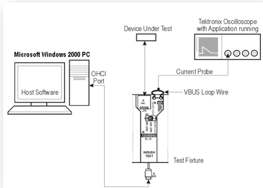
Figure 39: Equipment Setup for Full Speed Inrush Current Test
