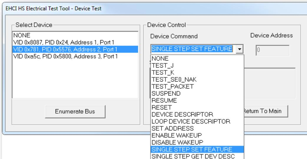
Figure 8: Device Single Step Set Feature
