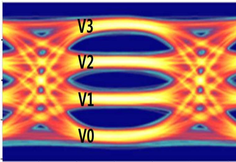
$V_0 \sim V_3$  is the mean value of the levels
