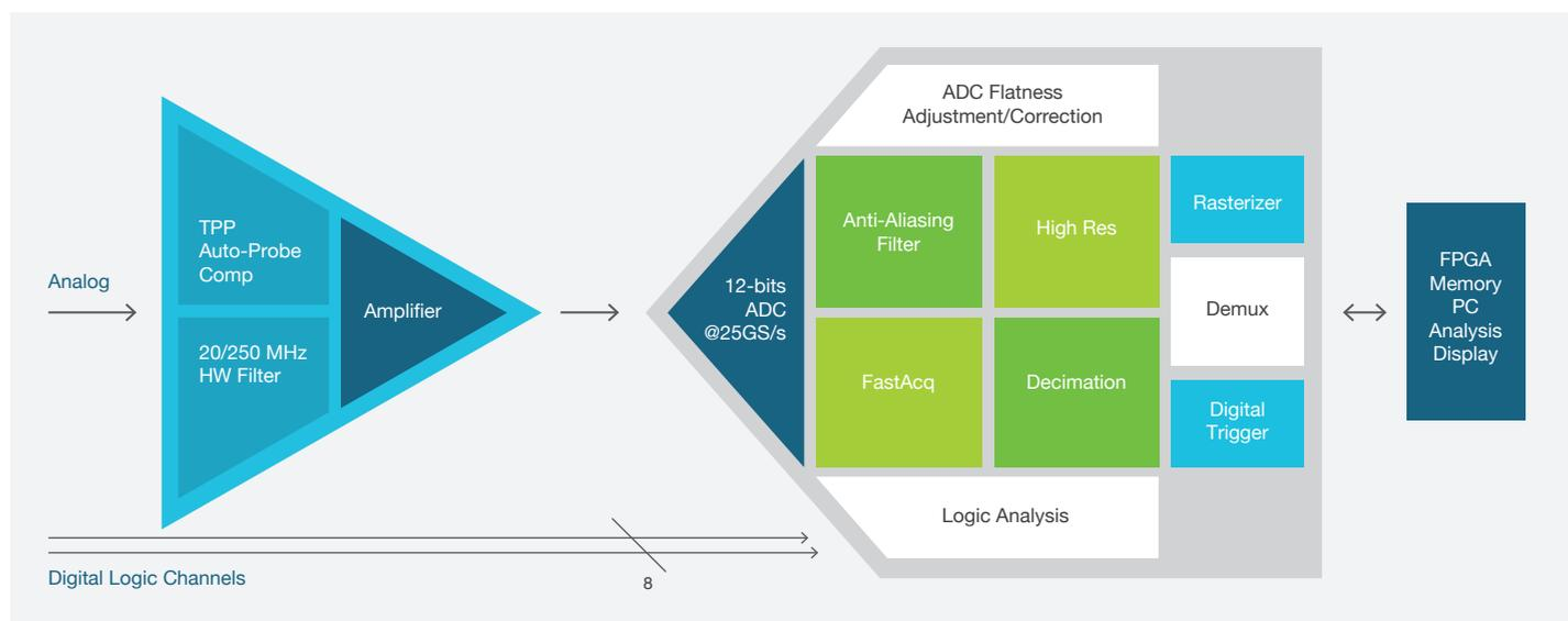
Figure 4: The 5 Series MSO acquisition path for one channel.
