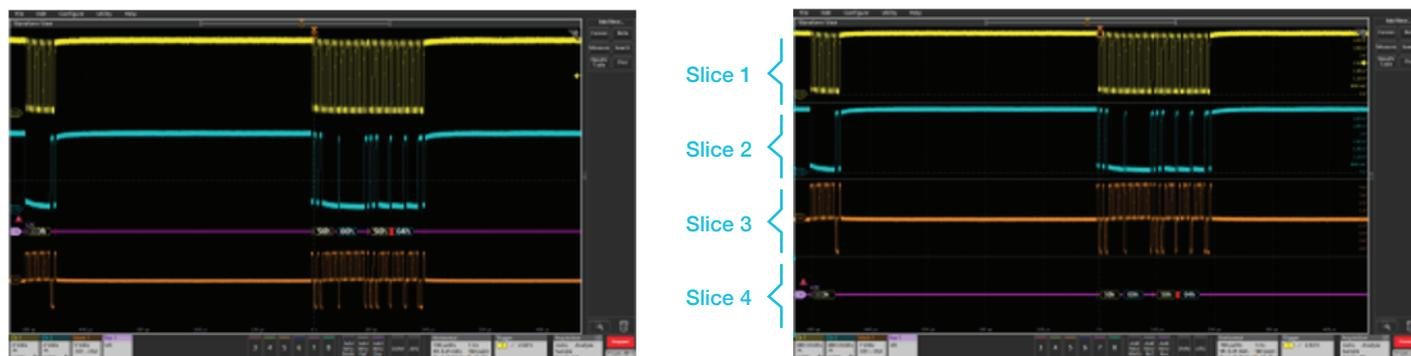
Figure 5: Each slice of the stacked display mode (right) can utilize the full range of the Tek049's ADCs, whereas each waveform in the overlay mode (left) uses only a fraction of ADC range.
