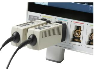
The internal power supplies of these oscilloscopes provide power to the TekVPI probe inputs located on the front of the oscilloscope (Channels 1, 2, 3, 4, Aux In, and RF). Because some of the available TekVPI probes can draw a significant amount of power, it is possible that multiple probes may exceed the oscilloscope's available internal power.
