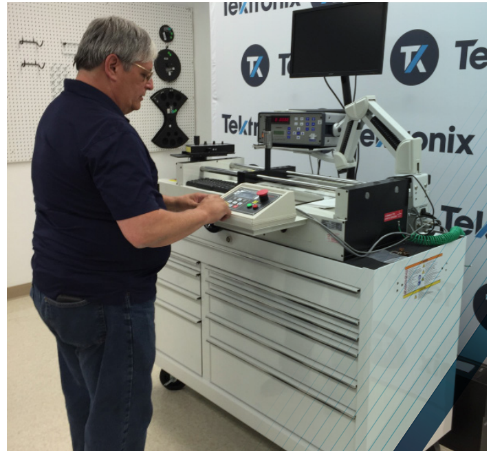
Fig 1 Tektronix Torque Calibration Station
