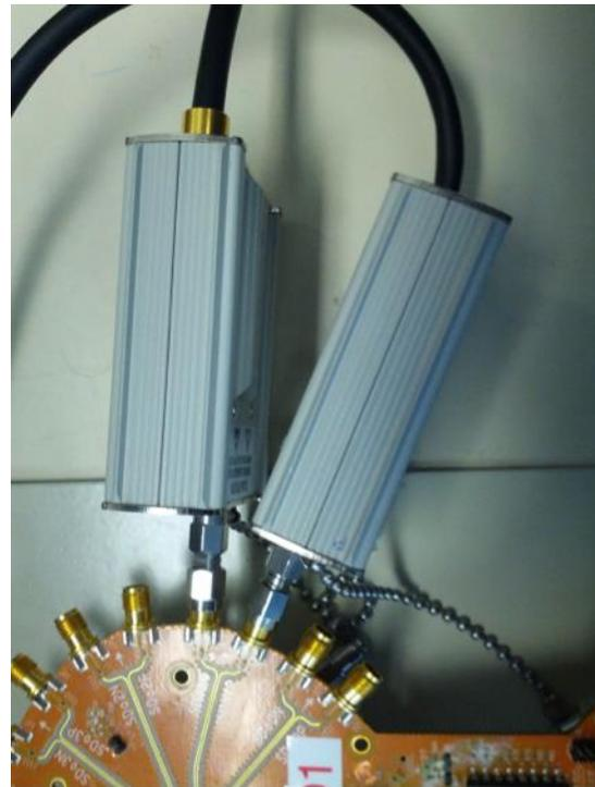
The remote heads and the 70 GHz oscilloscope bandwidth also provided the performance needed to handle the fast rise times on signals coming out of the device. This allowed for more accurate vertical noise measurements and cleaner eye diagrams such as seen in the screen shot below.
