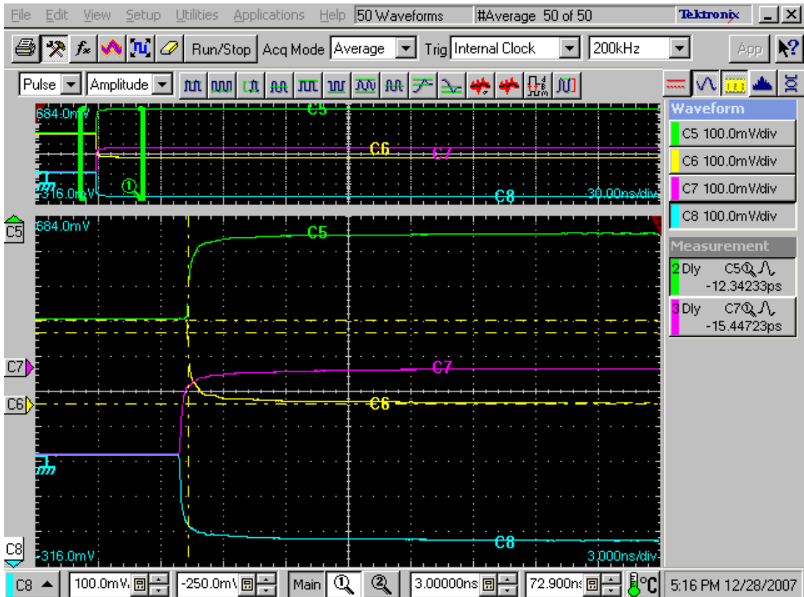
Figure 5.2.2. Delay measurements for inter pair skew calibration. The measured delays -12ps and -15ps for Port3 and Port4 respectively.
