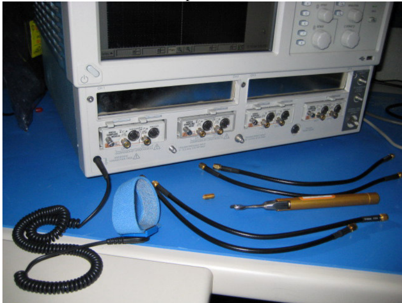
Figure 1: Equipment required to perform mixed mode deskew procedure. The wrist strap is important for ESD protection and a calibrated torque wrench is recommended to protect the connectors and to get good repeatability.
