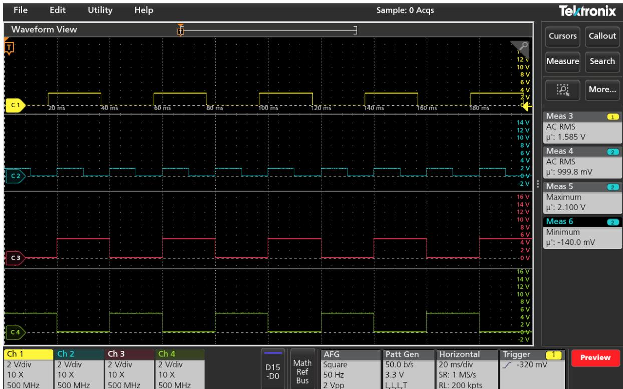
Figure 2. Waveforms from Task 1, step 6. Channel 1 is the data input, channel 2 the CLK, channel 3 is the  $Q$  output and channel 4 is the  $\bar{Q}$  output.
