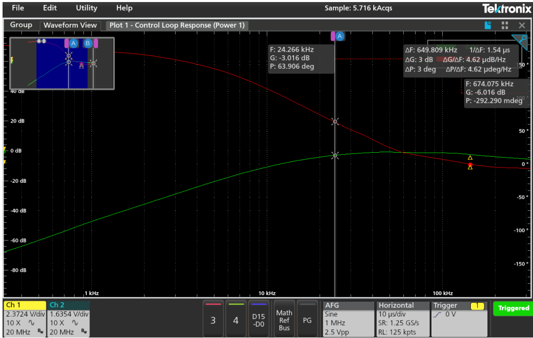
Figure 5. High pass filter bode plot results. Measure cutoff frequency of 24.266 kHz.
