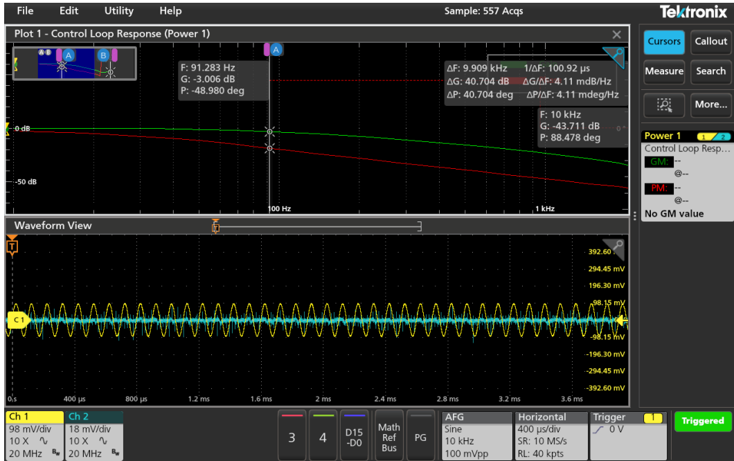
Figure 4. Low pass filter bode plot results. Measured cutoff frequency of 91.283 Hz.
