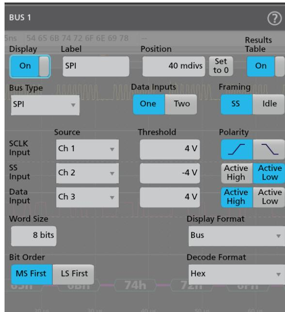
Figure 2. Bus configuration for SPI input.
