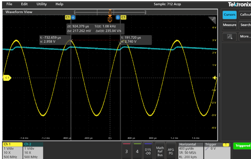
Figure 4. Expected waveforms from Task 2. V_{\text{ripple}} = 217 \text{ mV} , Frequency = 1 kHz.
