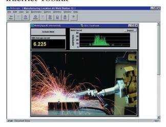
The Internet Toolkit provides the ability to view and control remote applications using an internet browser or TestPoint application. Remote sites can send email based on test status, or can communicate directly with any TCP/IP network client.
