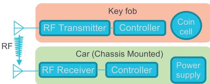
FIGURE 1. Remote keyless entry (RKE)/Remote start.
