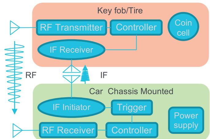
FIGURE 2. Passive keyless entry (PKE/Passive Start (PS)/Tire Pressure Monitoring system (TPMS).
