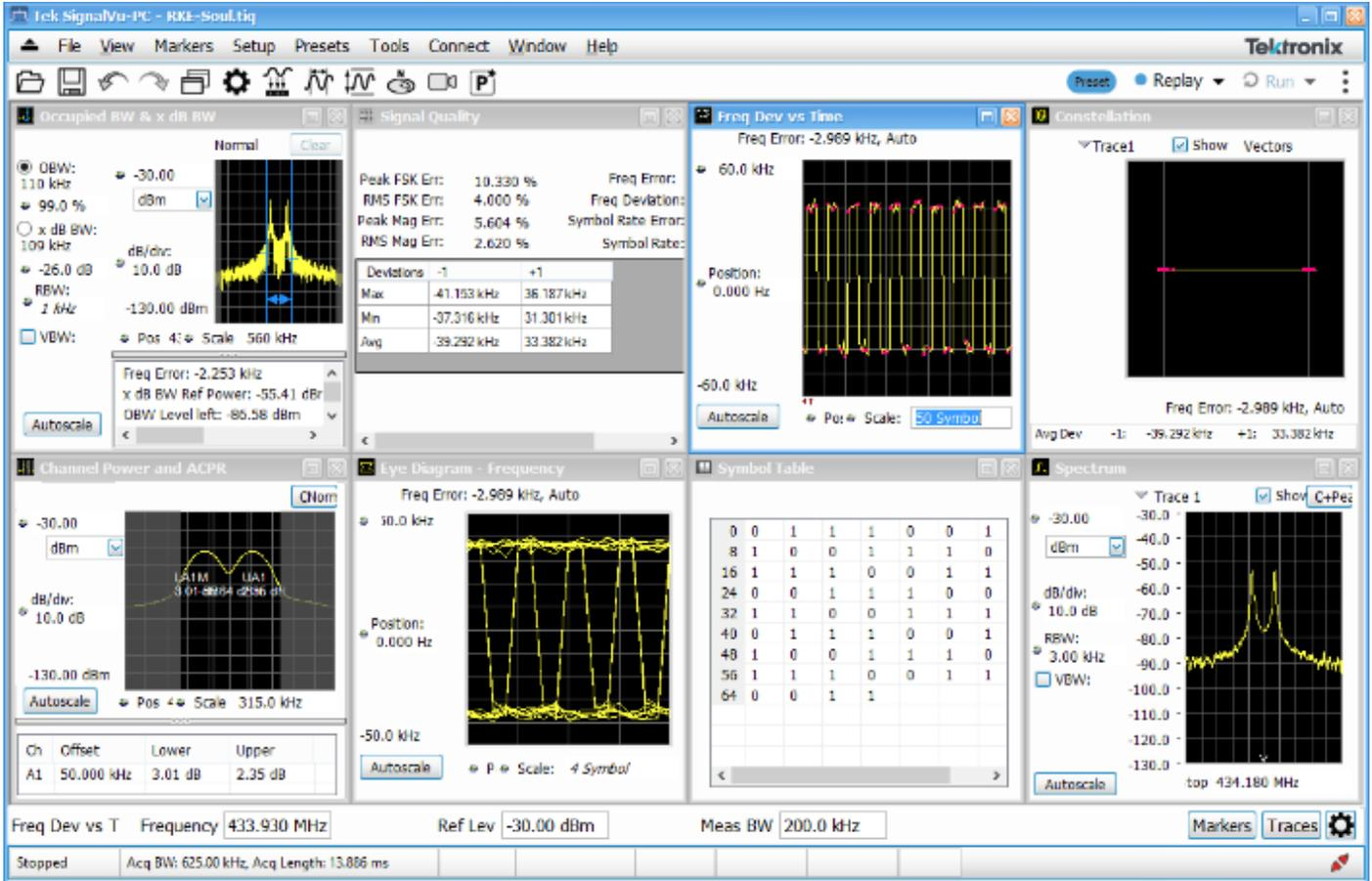
FIGURE 7. FSK analysis in Tektronix SignalVu-PC.
