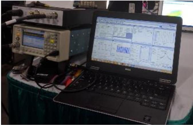
FIGURE 9. TSG4100, RSA600, and SignalVu-PC Software for TPMS transceiver tests.
