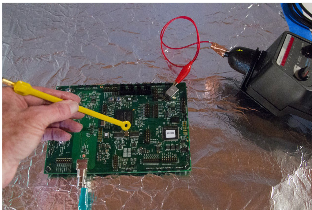
Figure 5. The ESD simulator is adjusted to a moderate voltage, such as 500 volts, and connected through the contact discharge tip to the demonstration board under test. The H-field probe is scanned around the board while observing the highest amplitude voltage peaks.
