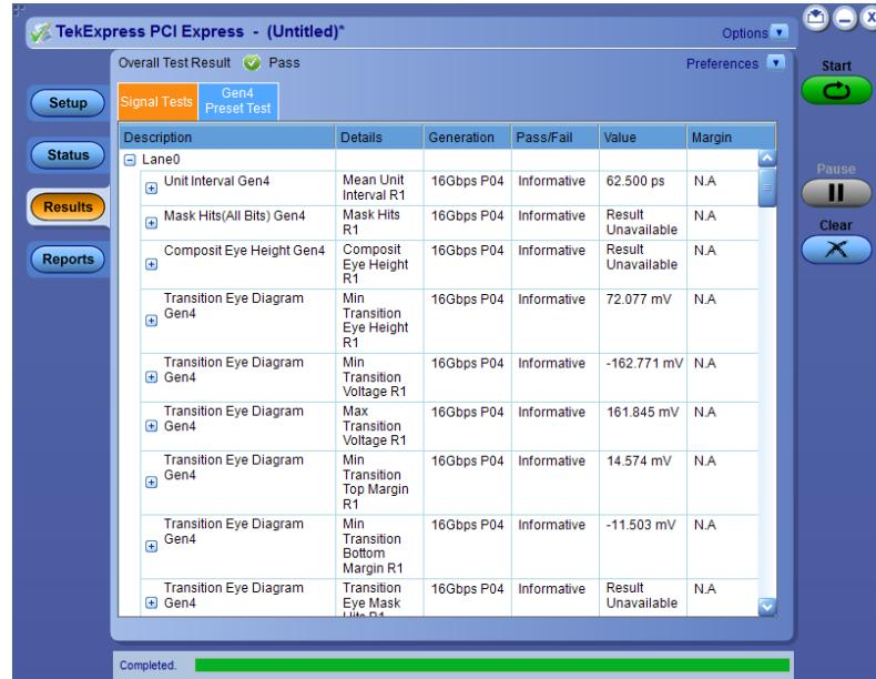
Figure 51 TekExpress PCI Express System-Board Signal Quality Test Results
