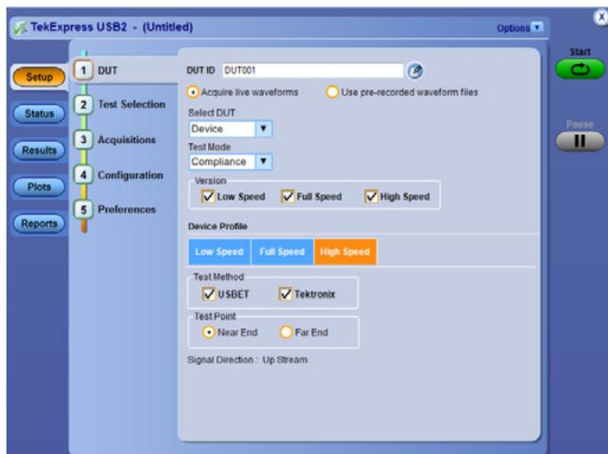
Figure 1. TekExpress USB2 High speed compliance software.
