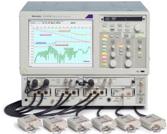
**Figure 23.** DSA300 Sampling oscilloscope with IConnect TDR/S-Parameter measurement software.
