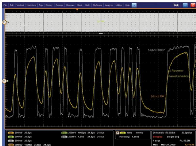
Figure 12. Hardware channel vs. Software emulation of 24 inch trace.
