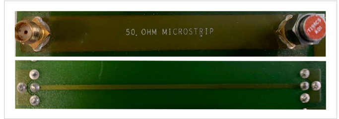
Figure 17. 50 Ω microstrip, top and bottom view.
