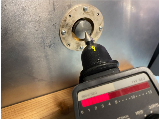
Figure 6. The contact discharge tip should be as centered in the target as possible prior to triggering the pulse.
