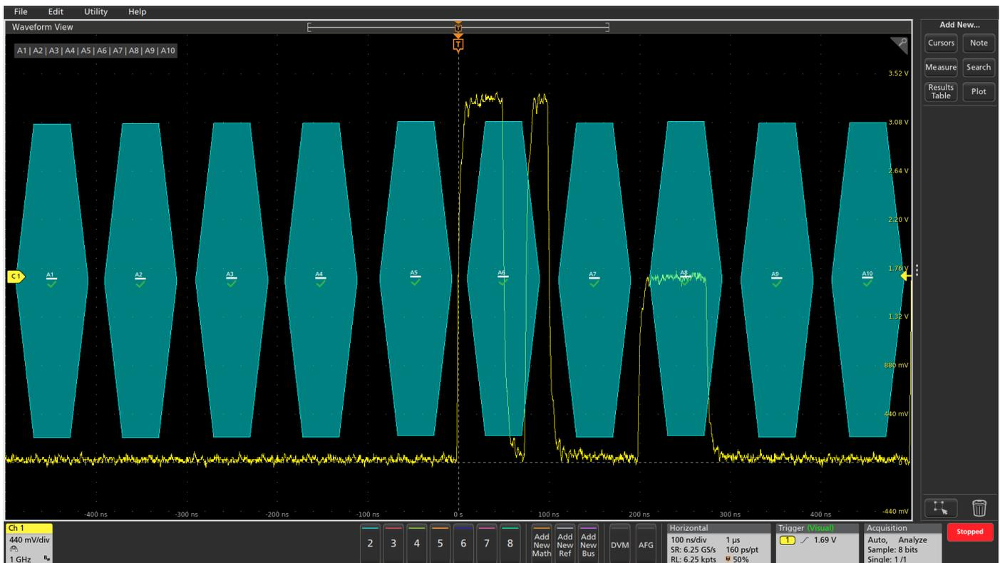
This example shows how Visual Trigger can be used in an unattended monitoring application to capture infrequent anomalies. First, a hexagonal area is placed in the center of each unit interval of this CAN signal. Then the logic equation is edited to logically OR all of the areas together. Finally, infinite persistence is used to capture all trigger events while the circuit is running for an extended period of time. Only the “mask” violations are captured.
