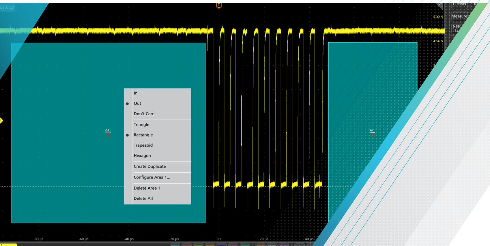
Capturing and finding the right characteristic of a complex signal can require hours of collecting and sorting through thousands of acquisitions for the event of interest. Defining a trigger that isolates the desired event and shows data only when the event occurs will speed up this process.
