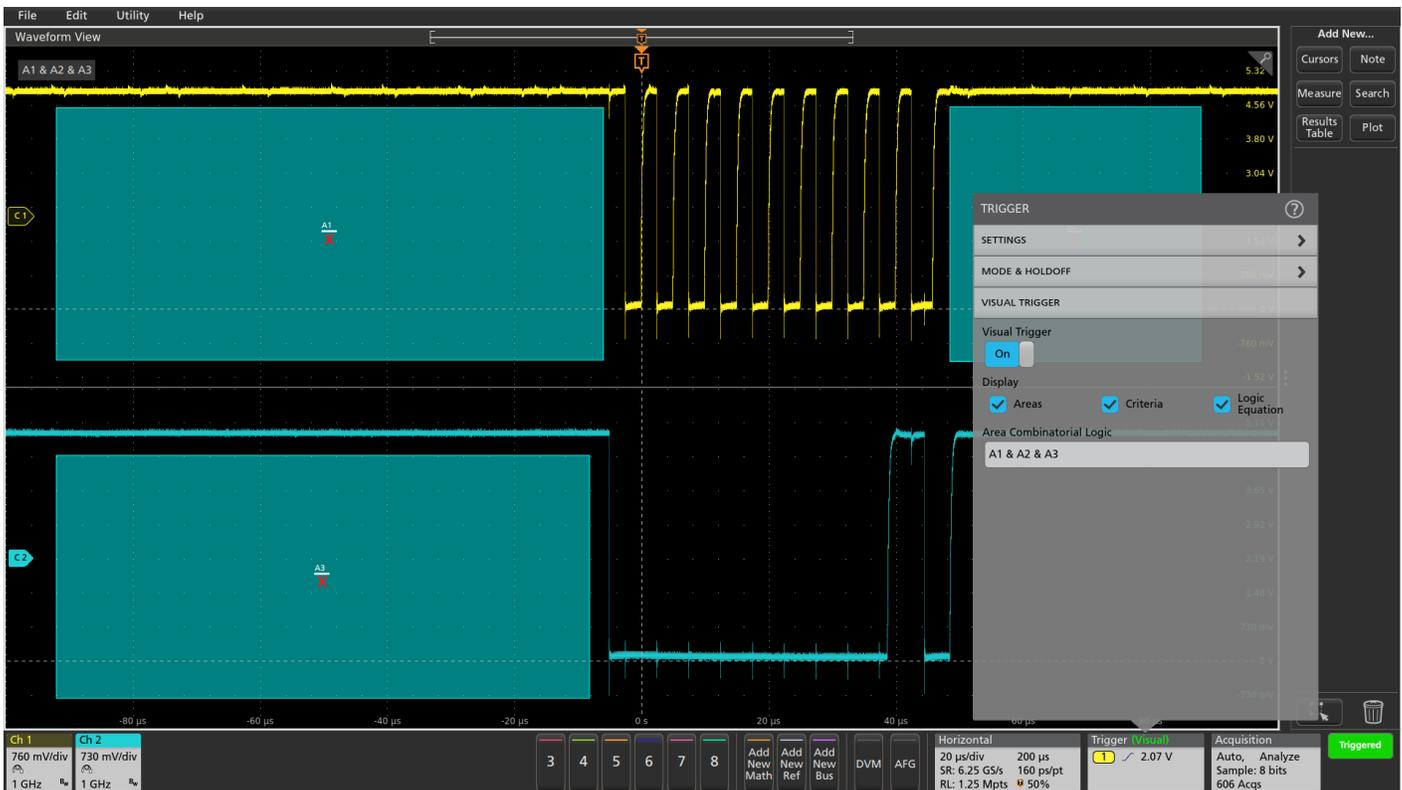
On the 5 Series MSO, and other scopes with the same user interface, Visual Trigger controls are found on the VISUAL TRIGGER panel in the Trigger configuration menu. Controls are provided to turn Visual Trigger on and off, customize the display, and enable editing of the Visual Trigger combinatorial logic equation. This equation describes how Visual Trigger will logically combine the areas to determine which acquired waveforms are displayed and which are discarded.
