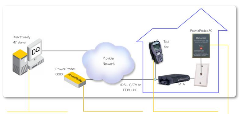
The DirectQuality R7 Server receives test requests from the technician's testset in the field, then immediately informs the PowerProbe 6000 to start the test.
