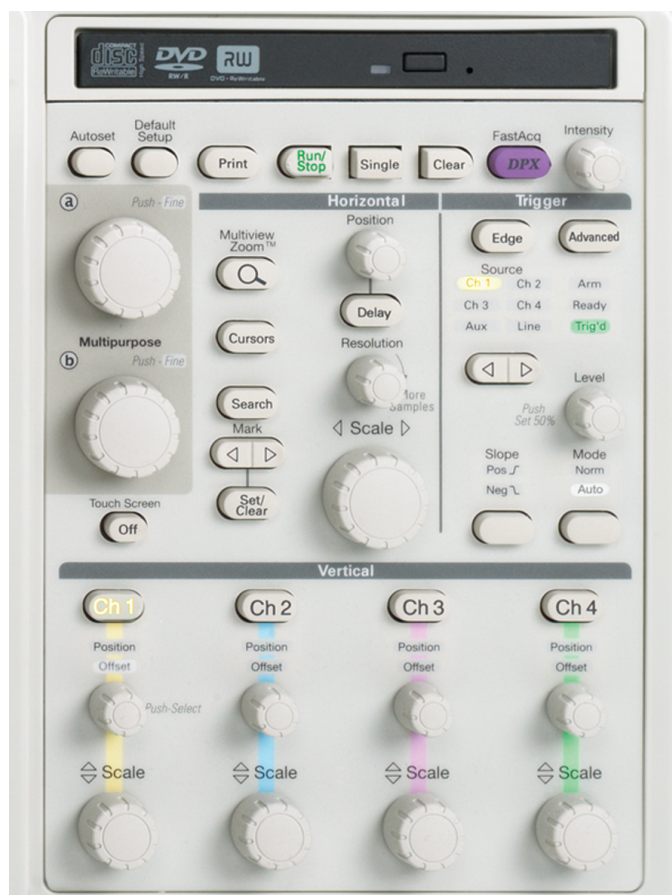
Figure 20. Front-panel control section of an oscilloscope.
