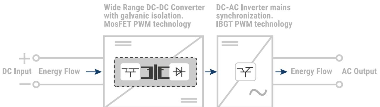
**Figure 7.** Electronic load DC output is applied to a grid-tied inverter stage.
