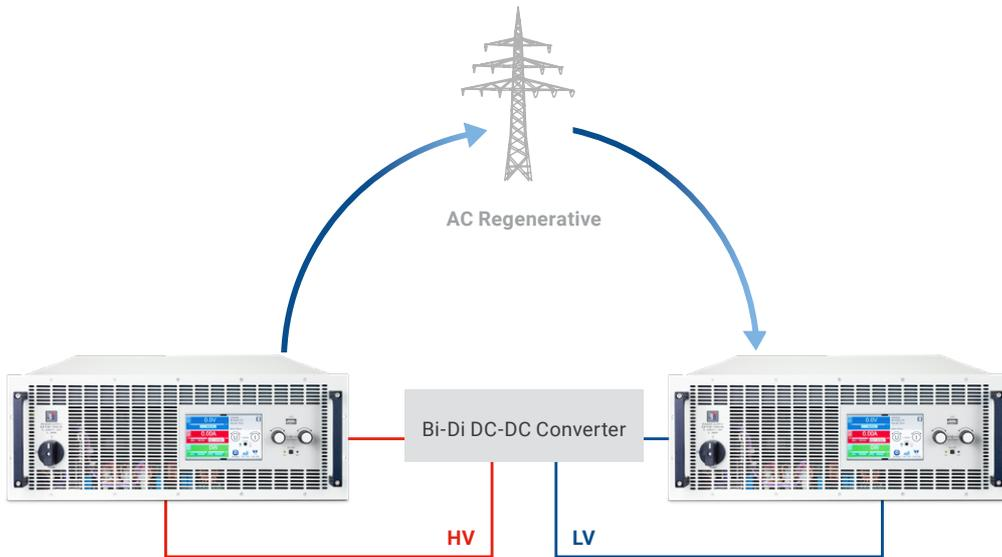
**Figure 9.** DC-DC converter test uses regenerative load to return 96% of energy back to its source.
