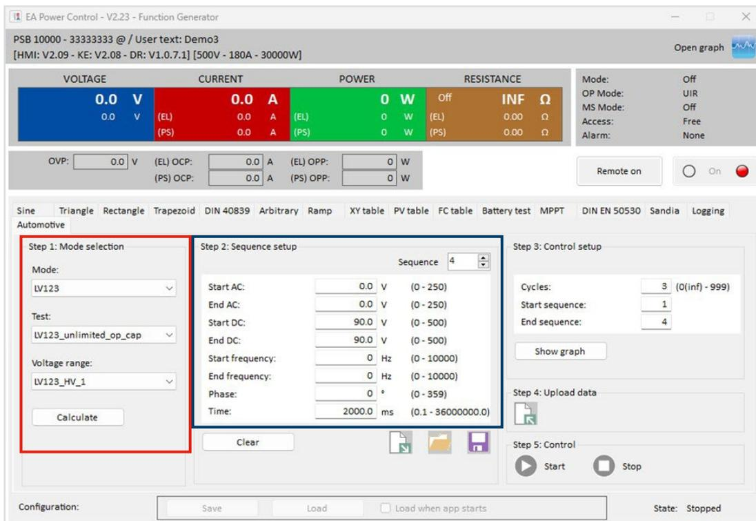
Figure 5. PC display presenting setup details for selected LV123 test profile.
