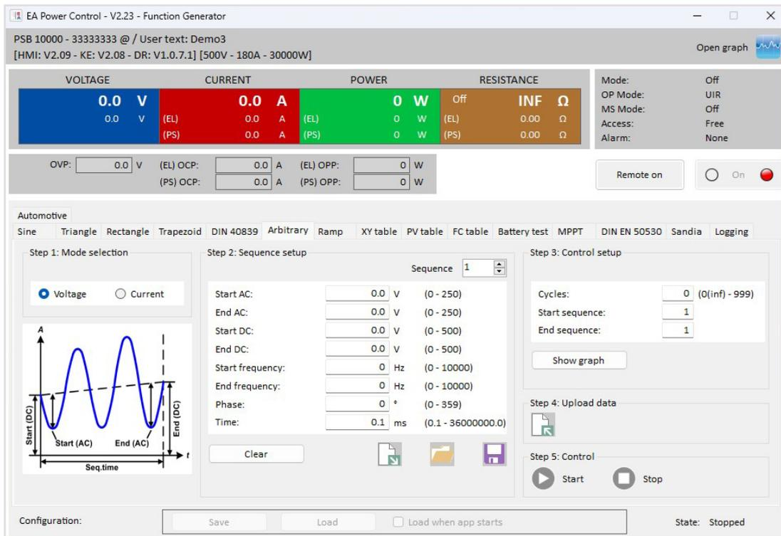
Figure 8. Arbitrary wave form generator used to profile load driven by the DUT output.
